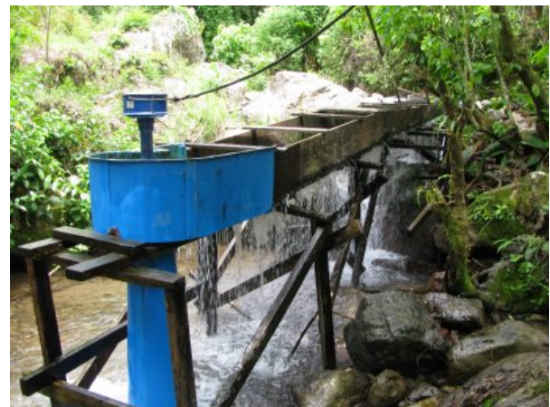
A pico hydro system made by the Sustainable Vision project from Baylor University [1]
