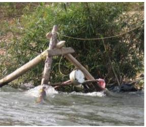
Figure 11 - Schematic figure 'lying' pico-hydro unit in River
