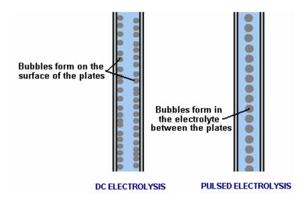
With straight DC-electrolysis, the bubbles of hydroxy gas form on the face of the plates and break away, helped by the thousands of microscopic, sharp-peaked mountains created on the face of every plate by the two-direction scoring with sandpaper. With the pulsed technique, the hydroxy bubbles form in the electrolyte itself, between the plates and give the visual impression of the electrolyte boiling.
