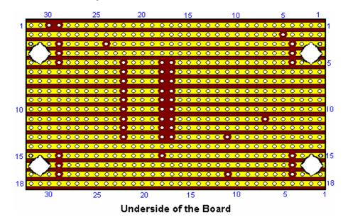
This shows where the breaks in the copper strips need to be made using a 1/8 inch (3 mm) drill bit.
