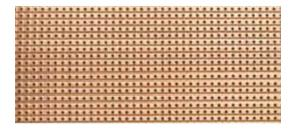
Strip-board (often called "Veroboard"), has copper strips attached to one side of the board. The copper strips can be broken where it is convenient for building the circuit. Component leads are cut to length, cleaned, inserted from the side of the board which does not have the copper strips, and the leads attached to the copper strips using a solder joint. Soldering is not a difficult skill to learn and the method is described later in this document.
