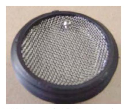
After fitting the mesh tightly into the cap, mount it with a 10/32 stainless steel saw on the opposite side to the 1/4" tapped hole for the barbed fitting. This is a flame arrestor, so make CERTAIN that the entire inside is covered tightly. Note that the sides wrap up. Turn each layer to cross the grain of the mesh.
