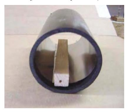
For drilling, use a strip of wood.
