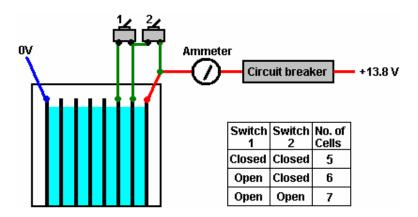
Here, the arrangement is very simple with two switches allowing one or two additional cells to be added in.
