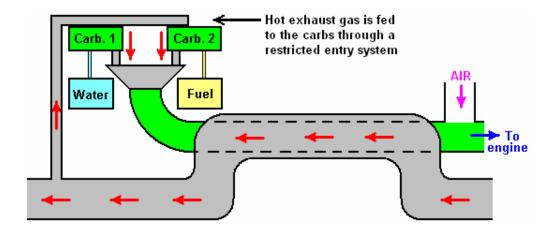
The use of carburettors is important since using a bubbler as suggested in the free plans on the internet, creates problems as the lighter fractions of the fuel get taken first which is exactly what we don't want to happen. The carburettors have the massive advantage that they feed all fractions of the fuel together and so the remaining fuel is always in the correct proportions.
