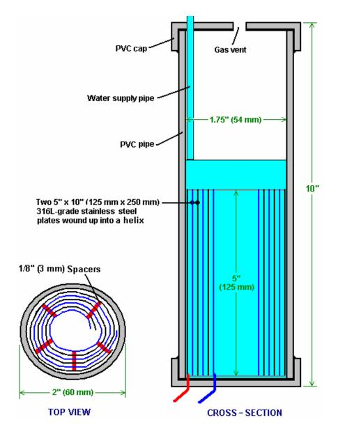
As the springy metal pushes outwards in an attempt to straighten up again, spacers are used to keep them evenly separated along their whole length by inserting 1/8" thick vertical spacer strips. The connections to the plates were made by drilling a hole in the corner of the plate, splitting the stranded wire, inserting the wire through the hole from both sides, turning it back on itself and making a wire-to-wire solder joint on both sides of the steel. The joint is then insulated with silicone.
