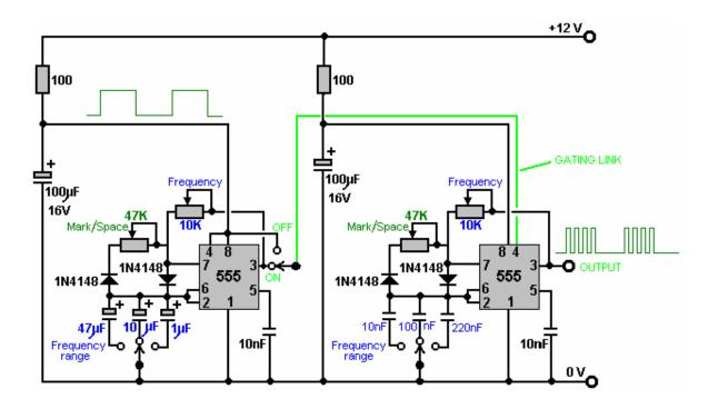
The final section of the circuit is the power drive for the electrolyser cell. This is a very simple circuit. Firstly, the output of the second 555 chip is lowered by a basic voltage-divider pair of resistors, and fed to the Gate of the output transistor:
