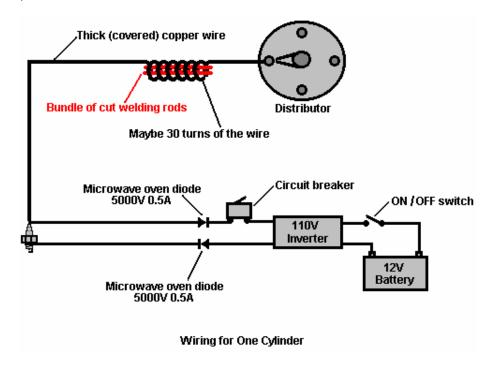
8. Be sure that the diodes going to the underside of the plugs are all the same way round and that the ones going to the circuit breaker are all the other way round as shown in the sketch. The other cylinders need to be wired like this:
