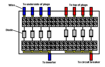
7. Run a 12-2 solid core wire from a diode to the underside of each plug. You can bend the wire round into a loop to fit tightly around the base of the plug, and then flatten the loop slightly with a hammer. The loop goes around the screw thread of the plug in a clockwise direction when looking down on it, so that turning the plug to tighten it, also tightens the copper wire loop. Alternatively, solder the open end of the loop to make it a rigid complete loop:
