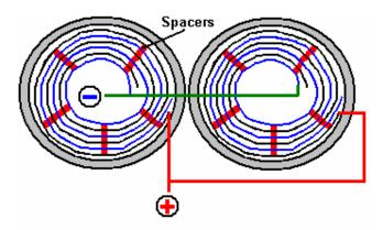
CELLS ARE WIRED IN PAIRS (Top View)
