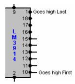
If the input voltage coming from the oxygen sensor is low, then all of these ten outputs will have low voltages on them. When the input voltage rises a little, the voltage on Pin 10 suddenly rises to a high value, while the other output pins still have low voltages.
