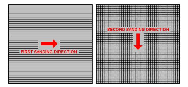
Bob Boyce uses a 6-inch x 48-inch belt sander which is great for preparing the plates and he uses it all the time now with 60 or 80 grit. Always wear rubber gloves when handling the plates to avoid getting finger marks on the plates. Wearing these gloves is very important as the plates must be kept as clean and as grease-free as possible, ready for the next stages of their preparation.
