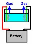
Here, a current flows through the liquid inside the electrolysis cell, moving from one plate to the other. The current breaks the bonding of the water molecules, converting the H<sub>2</sub>O into hydrogen H and oxygen O. There are various forms of hydrogen and oxygen and mixtures of the two. H atoms on their own are called "monatomic"
