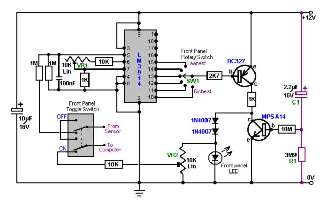
Electronic circuits are normally "read" from left to right, so we will look at this circuit that way. The first component is the 10 microfarad, 16 volt electrolytic capacitor. This is put there to help iron out any little variations in the voltage supply, caused by surges in the current drawn by the circuit when it switches from one state to another.
