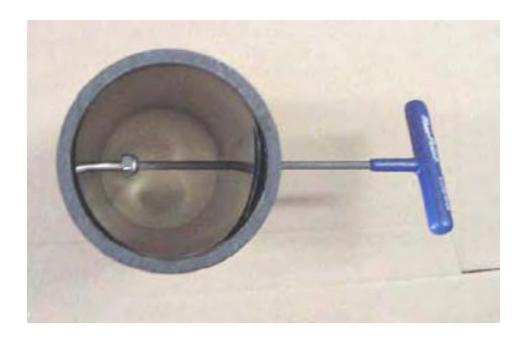
Note: This is why 2 holes are drilled (to facilitate assembly) Next, attach the electrode inside the barrel.
