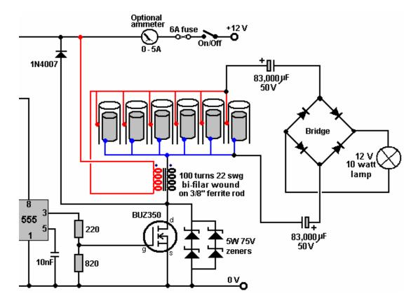
It has also been suggested that if a BUZ350 can't be obtained, then it would be advisable to protect the output FET against damage caused by accidental short-circuiting of wires, etc., by connecting what is effectively a 150-volt, 10 watt zener diode across it as shown in the above diagram. While this is not necessary for the correct operation of the circuit, it is helpful in cases where accidents occur during repeated testing and modification of the cell components.
