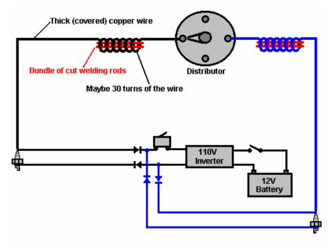
The wiring for two of the cylinders
