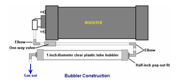
The elbows at the ends of the one-inch diameter bubbler tube have their threads coated with silicone before being pushed into place. This allows both of them to act as pressure-relief pop-out fittings in the unlikely event of the gas being ignited. This is an added safety feature of the design. However, it should be realised that the very high ignition rate of hydroxy gas creates a shock-wave which moves so fast that no pop-off fitting will ever be fast enough to rob it of its power.
