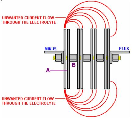
This diagram shows the way that the plates are connected. The red lines show paths of unwanted current flow which do not produce much gas. This wasted current flow is opposed by the useful current flow across gap "A" in the diagram.
