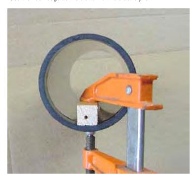
Clamp securely and drill two 0.165" holes, one on either side, perpendicular to each other, as best you can. These holes will be tapped 1/4" 20
