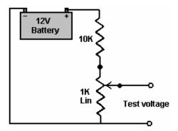
This gives us a voltage in the correct range when the shaft of the variable resistor is turned. Power up the circuit board by switching the 12 volt battery through to the board. Adjust the test-voltage source to 500 millivolts (0.5 volts) and apply it to the board's input (where the sensor connection will be made when it is installed in the vehicle). Set the switch to the "Richest" position, that is, with the switch connected to Pin 10 of the chip.
