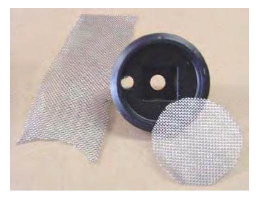
Next, prepare the stainless steel mesh. Cut it carefully to fit inside the threaded cap. Use at least 3 pieces.
