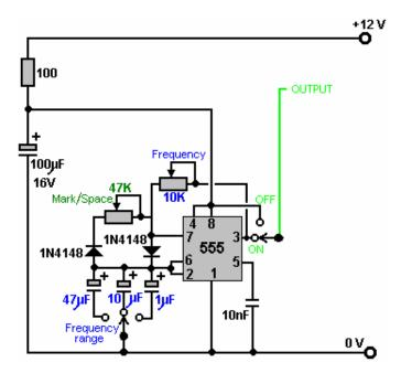
Which just has one additional switch to allow the output to be shipped and the 12-volt supply line to be fed instead. The reason for this is that this part of the circuit is used to switch On and Off an identical circuit. This is called "gating" and is explained in Chapter 12 which is an electronics tutorial.
