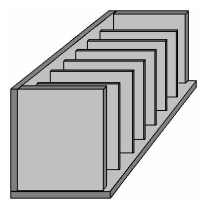
Here, the partitions are fixed in place one at a time, and finally, the second side is attached and will mate exactly as the partitions and ends are all exactly the same width. A simple construction for the Lid is to attach a strip all the way around the top of the unit and have the lid overlap the sides as shown here:
