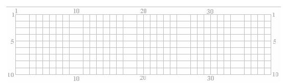
The horizontal lines represent the copper strips and the intersections with the vertical lines represents the matrix of holes. Many different layouts could be used for this circuit, so the following diagram is only a suggestion:
