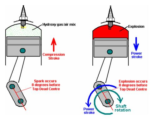
Here, the explosion is almost instantaneous and the explosion attempts to force the piston **dow nw ards**. Unfortunately, the crankshaft is trying to drive the piston **upwards** past the Top Dead Centre ('TDC') point, so the explosion will not help the engine run. Instead, the explosion will stop the crankshaft rotating, overload the crankshaft and connecting rod and produce excessive pressure on the wall of the cylinder.
