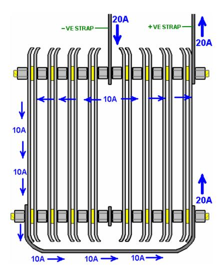
This arrangement is two identical sets of plates positioned back-to-back. To make it easier to understand the operation, let's just consider just one of the two sets of plates:
