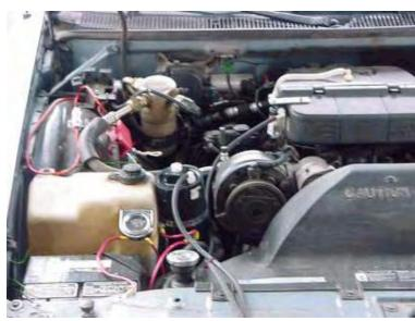
The unit draws only 15 amps which is easily handled by the existing alternator. The construction uses ABS plastic with Sodium Hydroxide ("Red Devil" Iye, 1 teaspoon to 8 litres of distilled water) and the gas-mix is fed directly into the air intake filter of the car engine. The electrodes are stainless steel with the negative electrode forming a cylinder around the positive electrode:
