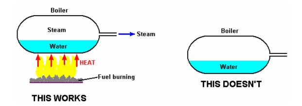
The power which drives the engine comes from burning the fuel. It does **not** come from the water, and in fact, if the engine were a Stirling engine, it would work perfectly well without any water being used at all. So, just to make sure this is clear, the power which drives a steam engine comes from burning a fossil fuel and the energy produced by that fuel burning could be used in various other ways which do not involve water at all.
