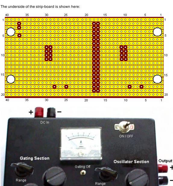
The ammeter shown here is not really necessary and can be omitted.
