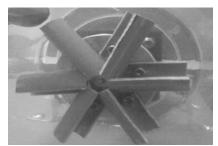
Fig. 7 Turbine for the proposed pico-hydro system
