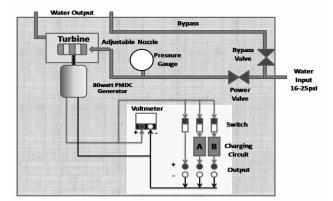
Fig. 6 Layout of the proposed pico-hydro system
