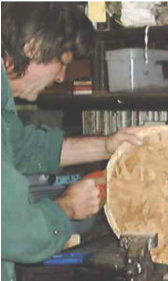
Sawing flat faces on the inner mould
