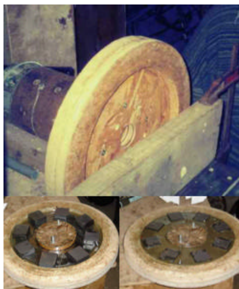
Rotor mould being made and used
