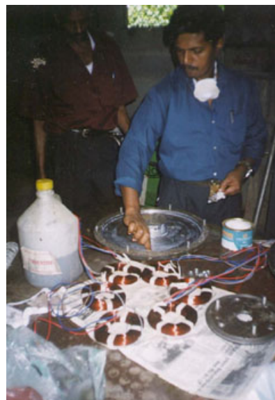
Figure 5 : making a PMG in Sri Lanka. Photo: Practical Action South Asia.
