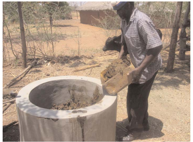
...to feed his biogas digester
