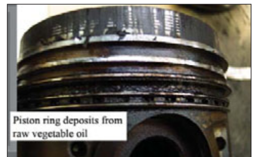
Figure 2. Deposits from raw vegetable oil
