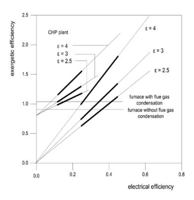
Figure A.4. Comparison of heat, CHP and power plant efficiencies by an exergetically weighted efficiency
