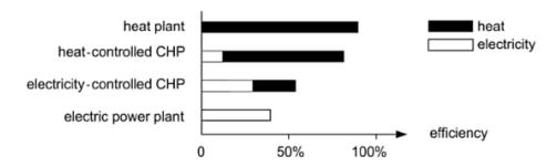
Figure A.3. Percentage of heat and electric power production in heating plants, CHP plants and power plants (qualitative figures)
