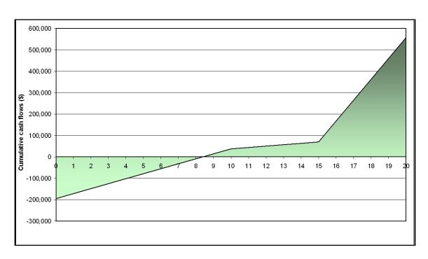
Figure 2. Cumulative cash flow (U\$) for: 500 cows herd, capital cost U\$ 9773/kW, fixed energy payment of U\$ 0.126/kWh for 20 years. Simple payback time: 8.5 years. Equity payback time: 8.4 years.
