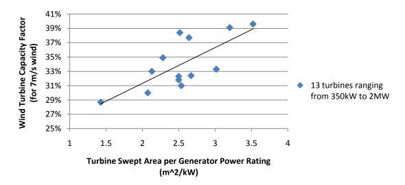
Figure 9: Capacity factor versus turbine swept area per generator power rating for 7m/s wind resource (see Table 19 and Table 20 for source data).
