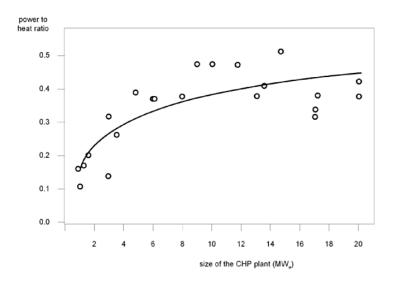
Figure A.2. Power-to-heat ratio as a function of the plant size of biomass-fuelled CHP plants in Finland and Sweden with 1-20MWe
