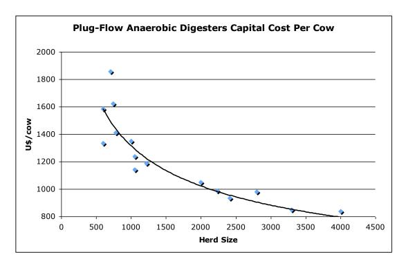
Figure 1. Plug-Flow anaerobic digesters capital costs = U\$ (16201 x number of cows^-0.3635) per cow (referred in this handbook as capital costs "level B")
