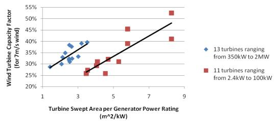
Figure 10: Comparison of Wind Turbine Capacity Factor to Swept Area per kW Rating for <100kW and >100kW wind turbines
