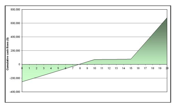
Figure 3. Cumulative cash flow (U\$) for: 1000 cows, capital cost U\$ 6320/kW, fixed energy payment of U\$ 0.070/kWh for 20 years. Simple payback time: 8.5 years. Equity payback time: 7.9 years.
