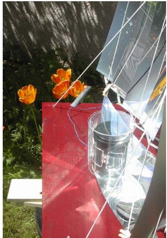
Figure 6. A polycarbonate windshield protects the cooking vessel.
