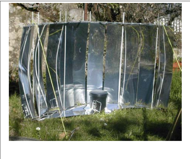
Figure 4. The following model works with a 3-dimensional fresnel geometry.
