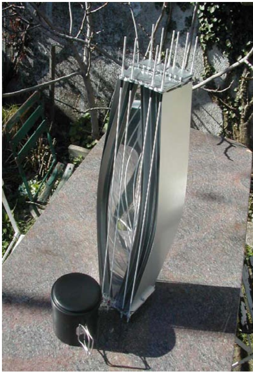
Figure 5. The 'scissor' mechanism allows for an easy folding of the cooker.
