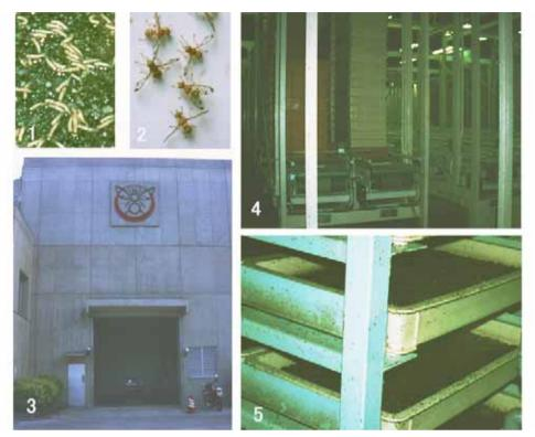
Plate 1. A plant producing sterile melon flies for their eradication: (1) larvae, (2) adults, (3) main building, (4) part of the automated rearing system, (5) feeding trays for larvae *(Courtesy Jun Mitsuhashi)*
