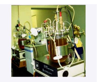
Plate 3. A model of a programmed cell culture system with glass jars (Courtesy Jun Mitsuhashi)
