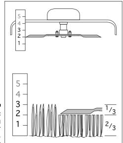
Figure 10-6: Setting mower height.
