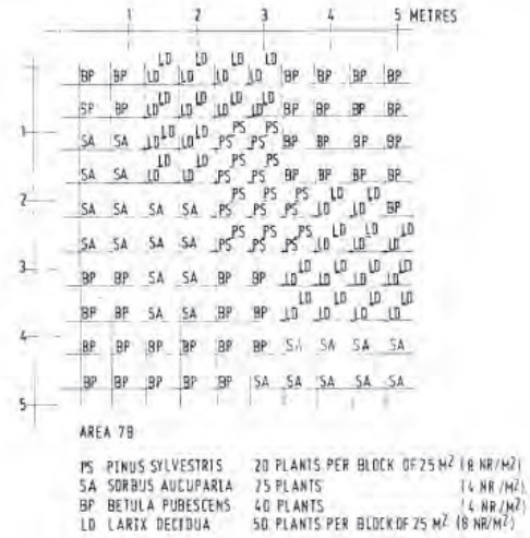
Figure 9.22 An example of a repeating unit for woodland planting. The setting out of units would be shown on a separate plan.
