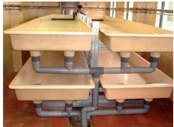
A trial version of a shallow raceway systems at a farm (A. Coelho & Castro) in northern Portugal.
