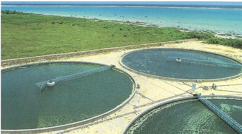
Figure 19. central pivot ponds used for the cultivation of Chlorella in Indonesia. Identical technology is used in Taiwan for Chlorella production.
