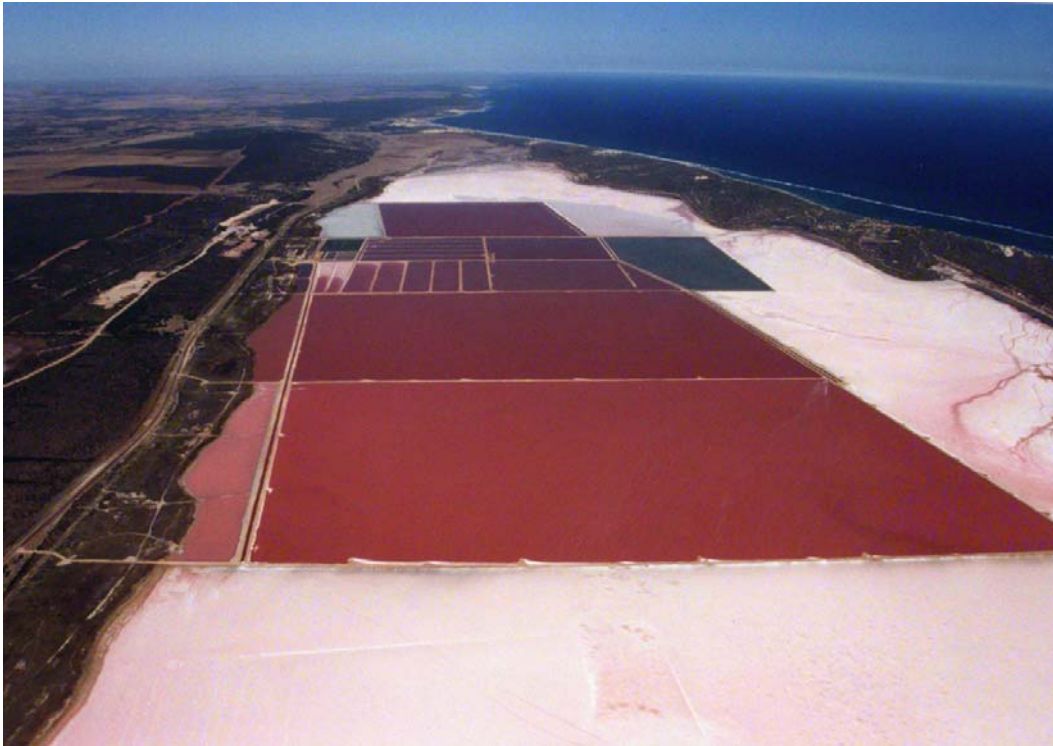
Figure 16. Dunaliella salina production plant at Hutt Lagoon, WA now operated by Cognis. Total pond area > 700 ha. This is the largest algae production plant in the world.
