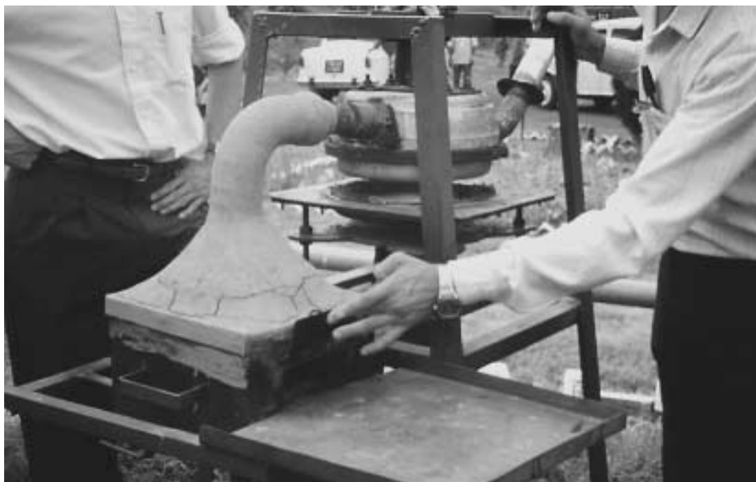
Photo 12. Non conventional energy press for mounding sal ( Shorea robusta ) plates at the Rural Development Centre, Indian Institute of Technology, Kharagpur, West Bengal. One of the key questions discussed during the workshop was how to launch viable enterprises of an appropriate size which do not keep people in low income activities.
