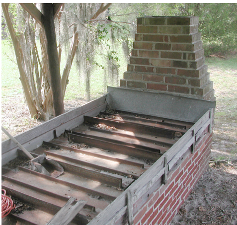
Evaporator with baffled pan and foam dipper for making ribbon cane syrup
