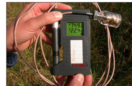
Above: A hygrometer can be used in the field to measure seed eRH and ambient conditions, informing post-harvest handling decisions.
