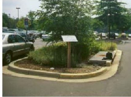
Photo 4 Rain-garden: This example receives stormwater from a car parking area (photo from ARC TP10 [3])
