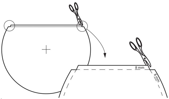
Put the larger piece of the circle on top of the sheet that you will use for the smaller piece. Align the edges and trace the relief cuts.
