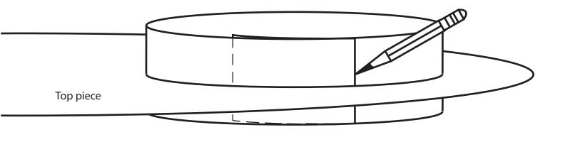
Make the strip flat again. From the mark you made, add 2 cm to make the piece longer. This 2 cm will be the tab. The tab needs relief cuts so that the edges of the strip can be folded.
