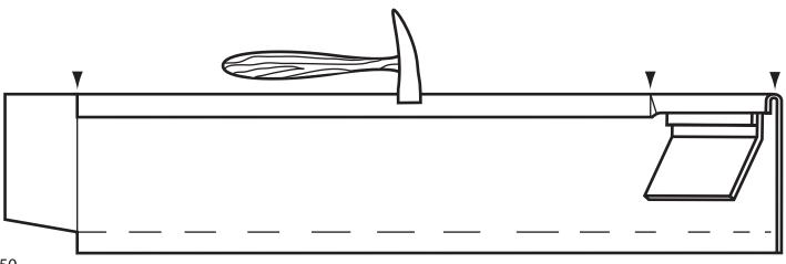
Bend the strip into a circle with the tab and the folded edge on the outside.
