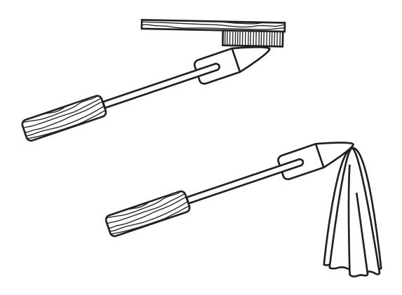
Heat the irons in the fire. When you heat the irons for soldering they should never glow red hot. This will damage the copper and waste time and charcoal.
