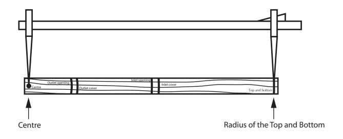
When the measurement is set, use the compass as shown in the illustration to find where to place the centre point of the circle.
