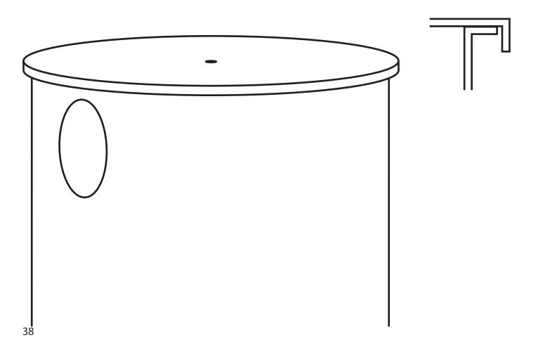
When you put them together they might not fit well at first. The body of the silo might not be a true circle. Mark with a pencil at the spots where it doesn't fit the bottom. Then gently tap it with the hammer from the inside. Only hit near the edge and be careful not to damage the soldered seams!
