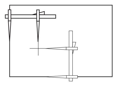
When the measurement is set, use the compass as shown in the illustration to find where to place the centre point of the circle. Don't scratch too hard or you will damage the galvanisation.
