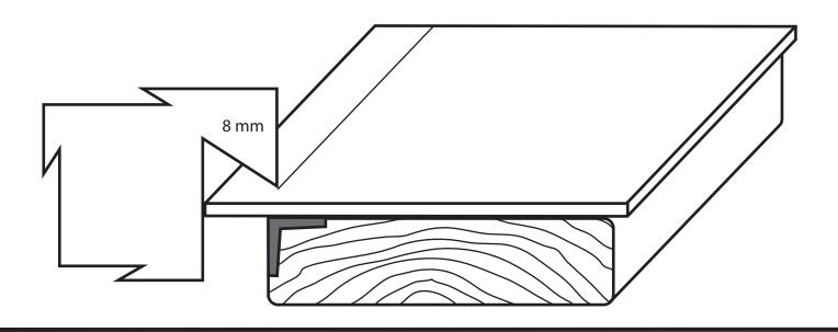
Use the wooden mallet and the edge of the bench with the angle iron to begin the fold.
