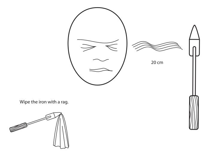
Rub the face of the hot iron in a shallow metal dish. If you are using resin then also add a little fine sand. Ammonium chloride is more corrosive than resin. It will cause the copper in the irons to deteriorate faster. Avoid breathing the vapours.
