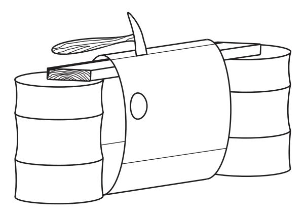
Solder the seams on one side of the sheet. The seam must be completely sealed with solder. The side with the solder will be the outside of the silo.
