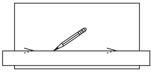
The marking gauge scratches a line parallel to the edge of the sheet. Here the gauge is used to make a line 12 mm from the edge. Hold the marking gauge 90 degrees to the edge of the sheet.
