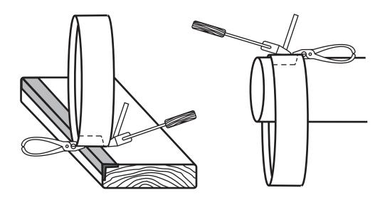
Use the marking gauge to mark 10 mm from the bottom edge. Make a small cut to the line about every 15 mm. Cut carefully to the line, not more, not less. This will help make a good joint.
