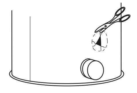
Cut a patch from scrap metal large enough to cover the hole plus about 2 cm extra all around. Use the acid to clean the metal. Solder the patch in place. Paint the solder joint inside and out as usual.
