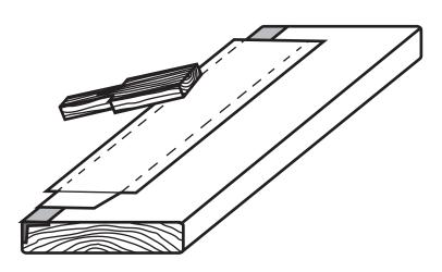
Use the hammer to close the fold but use the spacer for the last 3 cm on the end away from the tab.
