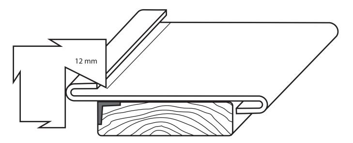
Use the spacer and the wooden mallet. Bend the edge to about 20 degrees on the bench. The edge must be bent away from the side with the fold.
