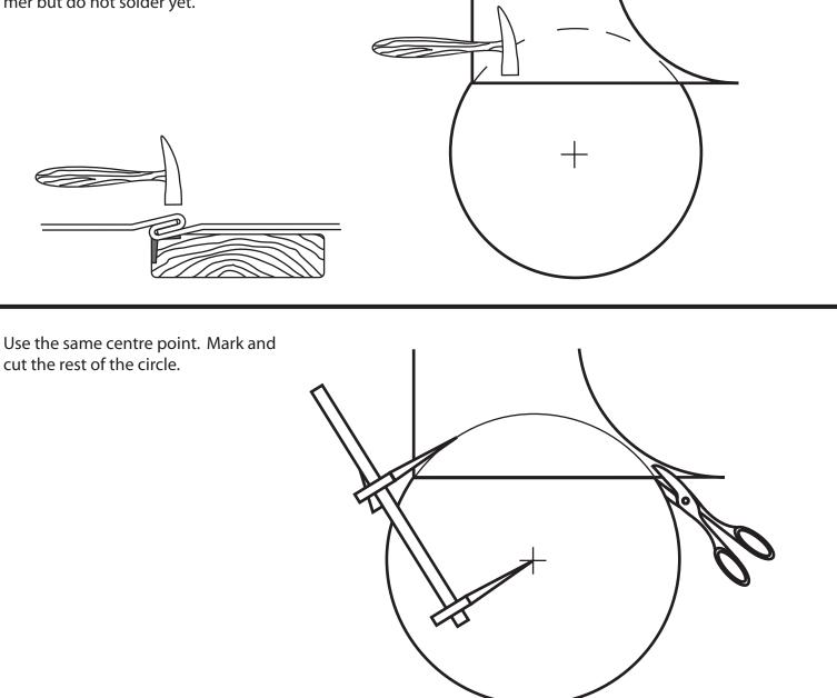
Solder only on the side that will be the outside of the silo. Put a drop of solder to cover the centre point of the circle.
