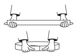
Place the strip in the hole in the top piece. Make sure that the long edges are lined up evenly. Make a mark where the end of the strip overlaps itself but don't cut it yet.
