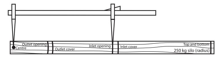
Using a story stick to set the compass for marking the hole for the inlet opening.
