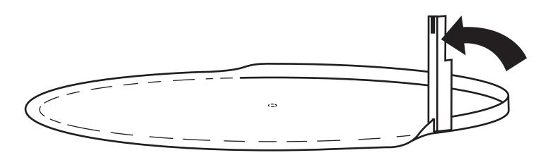
Put the bottom piece, flange down, over the body of the silo to see if they are the same shape.
