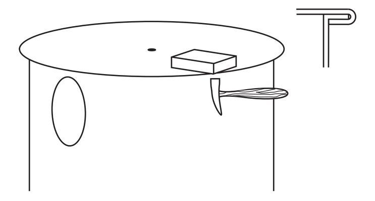
Turn the silo over. Solder around the flange. Be very careful not to leave any holes especially around the seams in the body.
