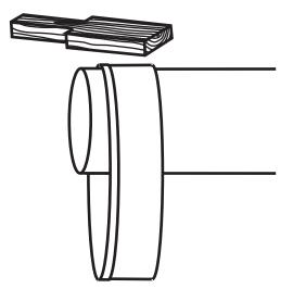
Use the flange method to join the top of the cover to the collar. Use the 8 mm bending tool.
