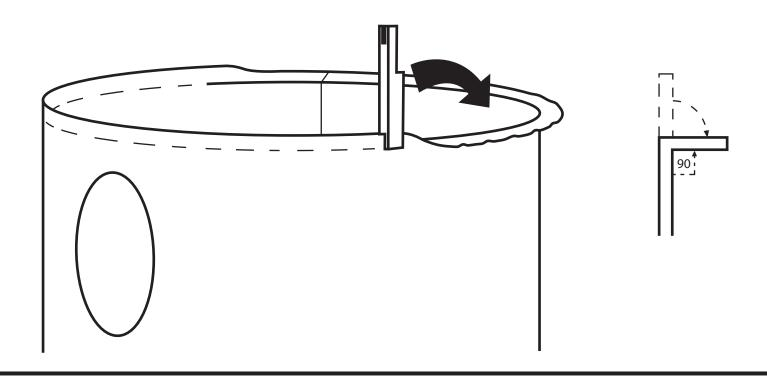
After using the bending tool, the flange will be wavy and uneven. Go around the edge carefully with the hammer and the counterblow to smooth out the flange. Stop when the flange is flat and even.
