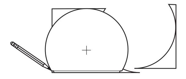
Use the seam method to join the pieces together.
