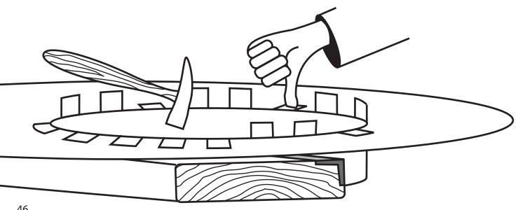
The top of the silo is now ready to be joined to the body. Use the flange method that you used to attach the bottom of the silo to the body.
