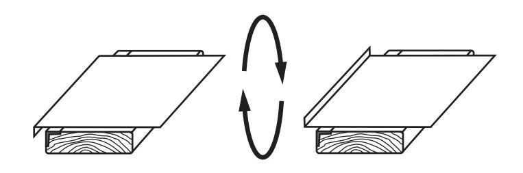
Use the spacer while you close the fold along the entire edge. At this point, the fold should be uniform and even.
