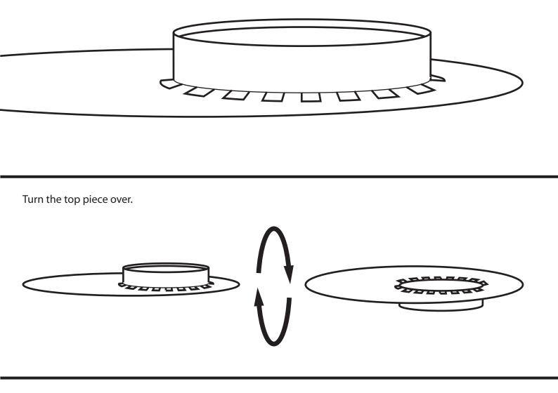
Bend some of the teeth to hold the opening in place. Go around the circle with the hammer and use the edge of the bench. Pound the teeth flat.
