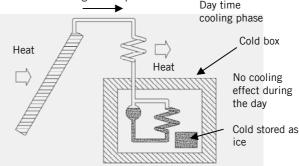
Heat phase: At high bed temperature and systems pressure, the refrigerant is driven out of the sorbent and collects in the cold box as a liquid
