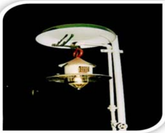
Biogas used for lighting of mantle lamps
