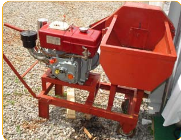
▲ This cracking machine is making it much easier for farmers to process the hard kernels of njansang.
