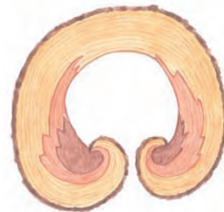
Figure 3.36. Diagram of decay in an inrolled crack.
