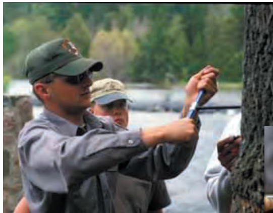
Figure 3.40-3.41. Invasive techniques may be used to quantify the extent of decay.
