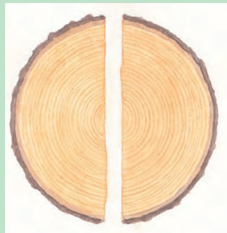
Figure 3.54. Cross section of a shear crack. The tree is split into two halves.
