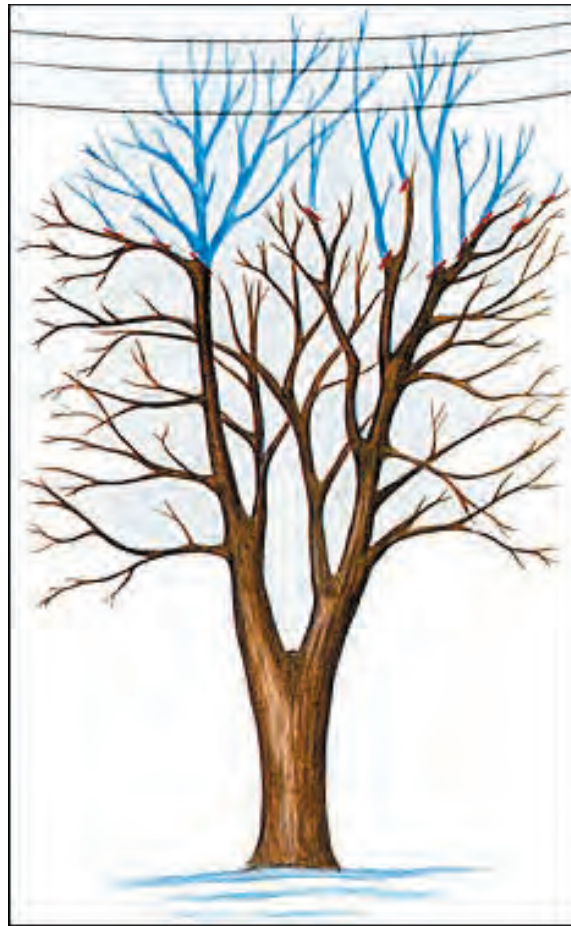
Figure 5. Crown reduction - branches to be removed are shaded in blue; pruning cuts should be made where indicated with red lines. To prevent branch dieback, cuts should be made at lateral branches that are at least one-third the diameter of the stem at their union.
