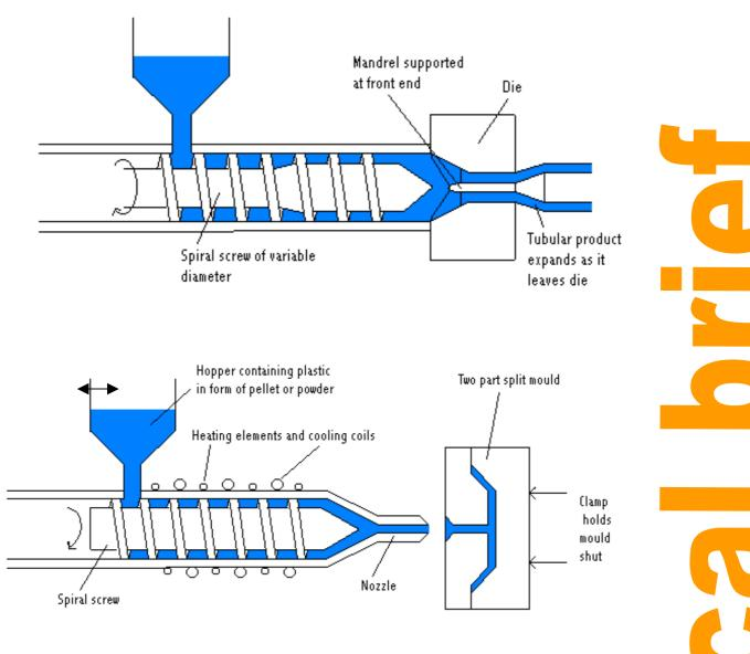
Figure 5: Plastic manufacturing techniques; extrusion (top), blow moulding (middle) and injection moulding (bottom).
