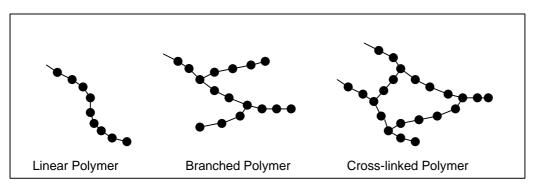
Figure 1: Polymer structures
