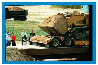
The composite bridge near Russell, Kansas, is load-tested shortly after its installation in 1996. Incorporating AOC resin technology, the bridge continues to pass load tests conducted periodically by the Kansas DoT.
