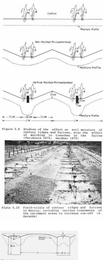
Figure 5.9 A proposed type of ridging for Botswana where a hard crust forms on the undisturbed ridges, giving higher run-off onto the cultivated strips
