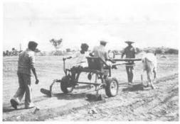
Plate 5.3 One of several tool carriers tested at ICRISAT for forming and cultivating beds (ICRISAT)
