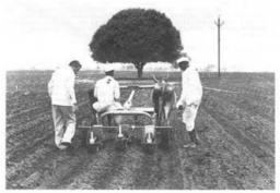
Plate 5.7 Trials at ICRISAT of a 3-row planter on broad beds (ICRISAT)
