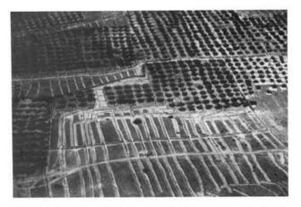
Plate 5.27 In the Sousse region of Tunisia, collecting drains ('meskats') lead run-off down to olive groves (J. Damagnez)
