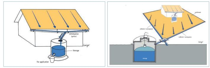
Figure 9: (left) water harvested from roofs used for drinking, domestic purposes and irrigation of kitchen gardens; (right) rooftop and courtyard water harvesting for irrigation of kitchen gardens and domestic use.
