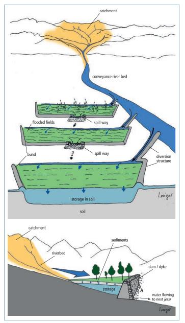
Figure 6: Floodwater harvesting; above: floodwater diversion system (off-streambed); below: floodwater harvesting within streambed, a cross-section of a jessour system. (jessr=singular).
