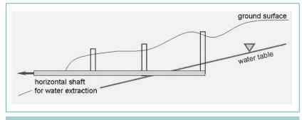
Description of a *qanat* system: Vertical shafts called mother wells (up to 50 metres deep) are dug close to underground springs or water table. Further, several and at more or less regular intervals "ventilation shafts" are dug in a straight line to target (Safriel and Adeel, 2005).
