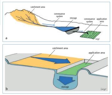
Figure 4: Basic componens of two WH systems: a) catchment area, storage and application area are clearly separated and connected by conveyance systems; b) catchment area is bordering application area. Storage is in the soil or ground below the application area with no need for extra conveyance systems.
