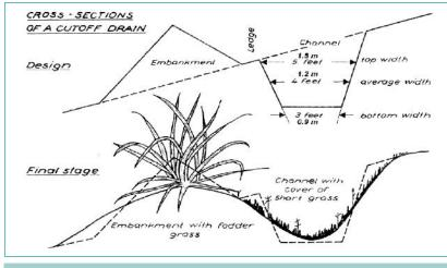
Cross-sections of a cutoff drain (Jaetzold and Schmidt, 1983).
