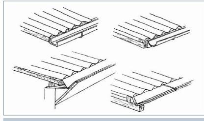
Square-sectioned, semi-circle, and V-shaped guttering with two different ways of attachment to the catchment area (Worm and Hattum, 2006)
