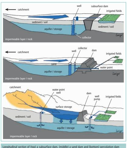
Longitudinal section of (top) a subsurface dam, (middle) a sand dam and (bottom) percolation dam (adapted from Foster and Tuinhof, 2004; Oweis et al. 2012).
