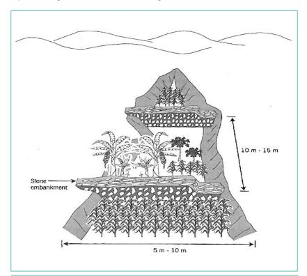
Stone enbankements slow down runoff, encourage sedimentation of organically rich deposits and create a moist and fertile gully bed, suited to crop production. Bananas, pawpaws and annual crops are planted between the stone checks (Mutunga and Critchley, 2001)
