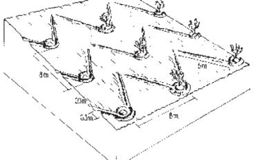
V-shaped micro-catchments which harvest water for the olive trees: the furrows up-and-down slope help channel the runoff to the olives. (Mats Gurtner)
