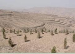
Large-scale application of microcatchments in China. (HP. Liniger)
