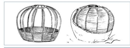
Construction of a water jar with a frame of iron bars or bamboo sticks covered with cement (Worm and Hattum, 2006).
