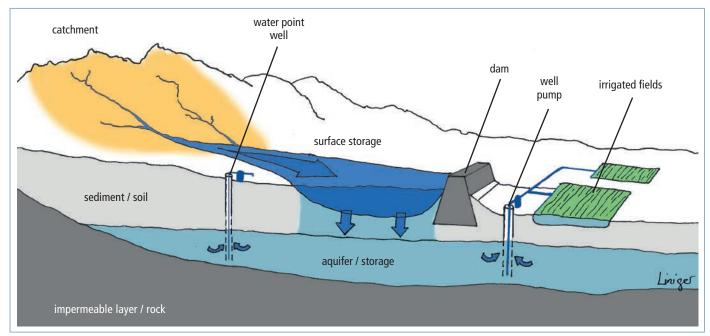
Figure 7: Macrocatchment water harvesting: a cross-section.
