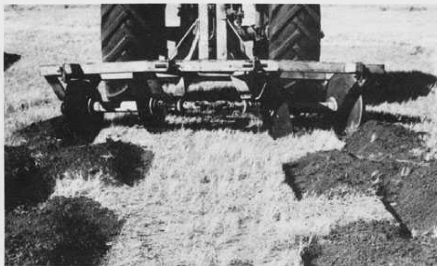
Figure 7.2 A modified disc plough for making pits on range land
