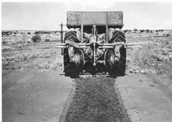
Plate 7.8 Opposed discs with ripper and grass seeder (Western Australia Department of Agriculture)
