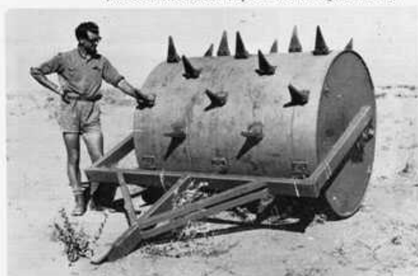
Plate 7.11 A spiked roller for range improvement, which can be filled with water to provide extra weight if necessary (Western Australia Department of Agriculture)
