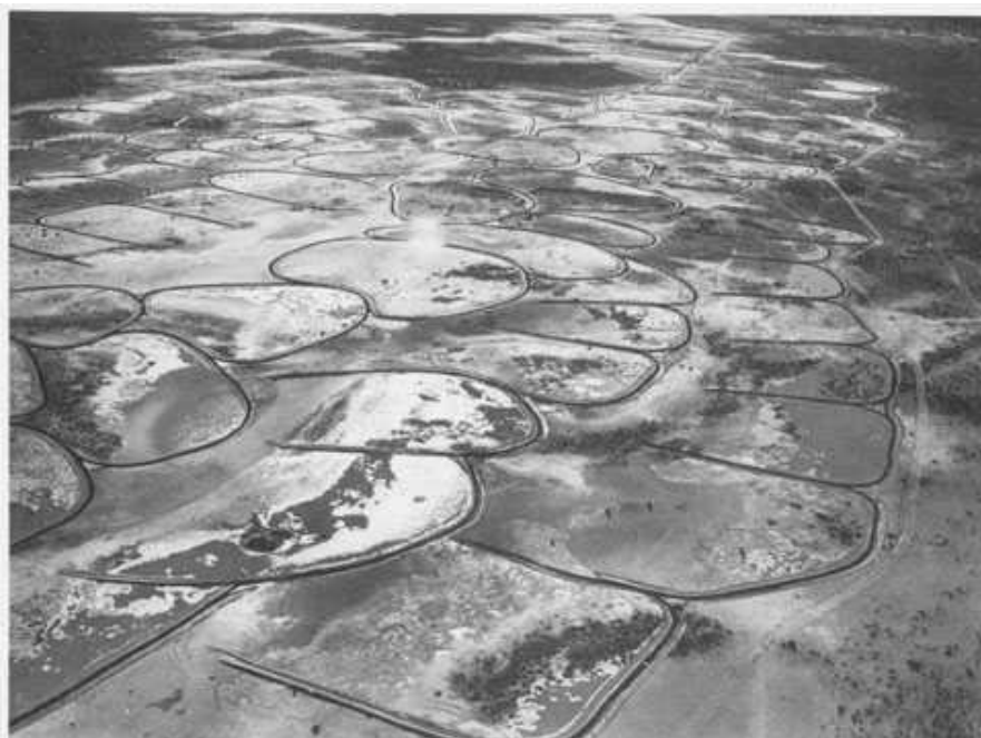
Plate 7.17 Ponding banks to leach salinity and encourage re-vegetation on 'scald' (Soil Conservation Service of New South Wales)
