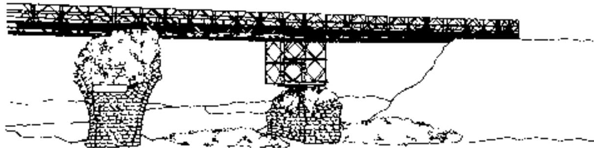
Figure 16-1. Continuous-panel bridge supported on damaged masonry pier and a panel crib pier
