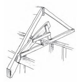
**8.21** Scissor prop to support the underpurlin in the absence of a wall onto which a strut could be fitted
