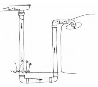
$\label{eq:Figure 9.7} \mbox{ Figure 9.7 Sealed PVC water transport from the roof to a water tank}$
