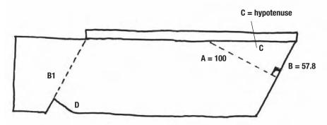
Figure 8.13 Transfer the calculated details to the roofing boat. B1 = vertical birdsmouth line. D = Top plate horizontal birdsmouth
