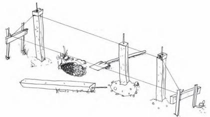
Figure 3.3 String lines for the installation of concrete stumps
