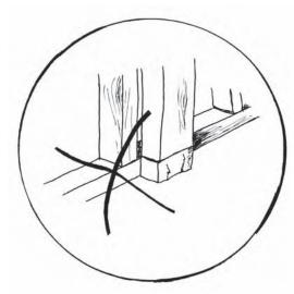
Figure 6.6 Incorrect installation of a short length of bottom wall plate beneath a door stud
