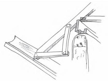
Figure 9.5 Soffit bearer to carry eave lining
