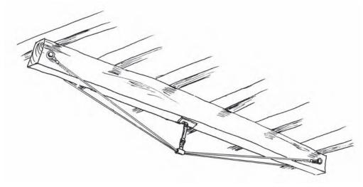
Figure 8.20 Tie-bolt or barrap truss
