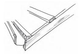
Figure 9.6 A tilt batten at the tail of the rafter as an alternative to fascia
