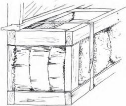
Figure 5.12 Timber framing for a timber-lined window seat
