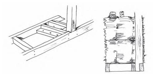
Figure 4.17 Connection of a structural infill post to the bottom boxing
