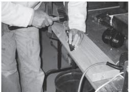
Figure 14.7 Clean up the checkout for the hinge using a sharp chisel
