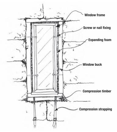
Figure 10.2 Fixing a window into a wall
