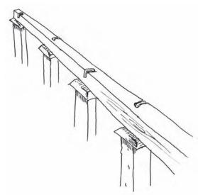
Figure 3.7 Pins of concrete stumps are bent to the left and right of the bearer
