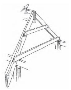
**Figure 8.16** Coupled roof with collar tie, ceiling joist and non-load bearing ridge
