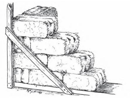
Figure 4.5 The use of a corner bale guide will help to keep the corner bales vertical and in line
