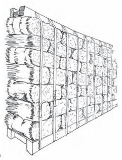
Figure 4.1 Basic straw bale wall construction
