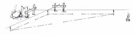
Figure 2.6 Marking the position of the wall at a right angle to the first wall
