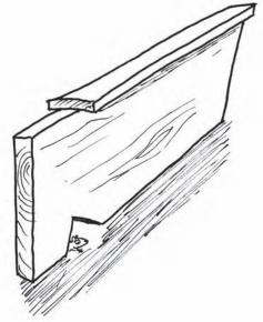
**8.12** Roofing boat used to mark timber to be cut for rafters
