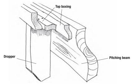
Figure 5.13 Dropped rolled head dropper joining the top boxing and pitching beam for infill construction
