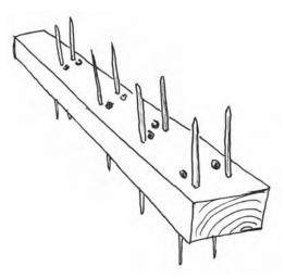
Figure 4.22 Spiked peg for installation between the rows of bales
