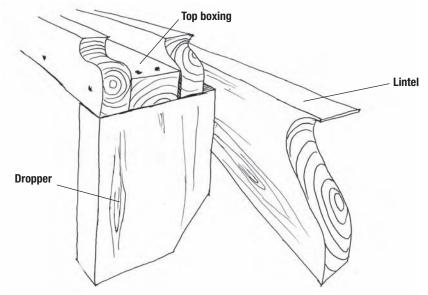
Figure 5.14 Dropped rolled head dropper joining the top boxing and window lintel for load bearing construction
