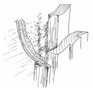
Figure 10.5 Architraves at the stile of the window to conceal the junction of the window and the render
