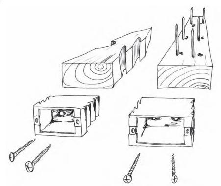
Figure 12.2 Barbed wooden peg to be hammered into the bale wall onto which the electric wall box is secured
