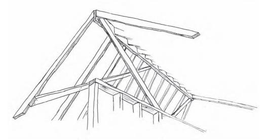
Figure 8.32 Two alternative methods of bracing a gable roof
