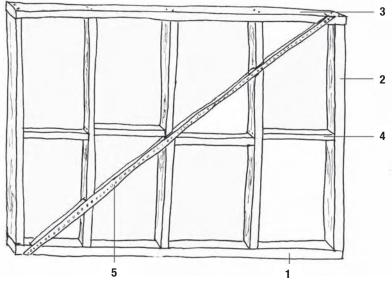
Figure 6.1 Simple timber framed wall
