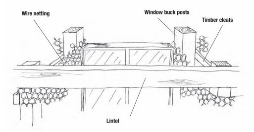
Figure 5.15 Wire netting over posts and frame of window buck for an externally located window with a pitching beam installed level with the internal wall
