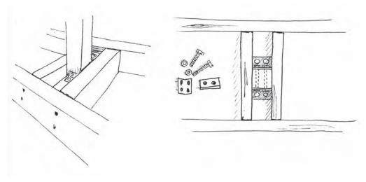
Figure 4.18 Infill post secured to the floor using metal brackets
