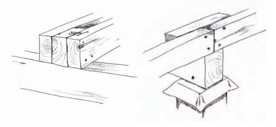
Figure 3.9 Insert stabilising blocks between double joists
