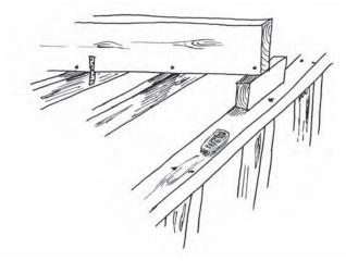
Figure 7.5 Installation of a supporting block between the hanger and the top of the wall
