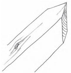
Figure 8.29 Double 45-degree angle cuts for the top of the hip beam
