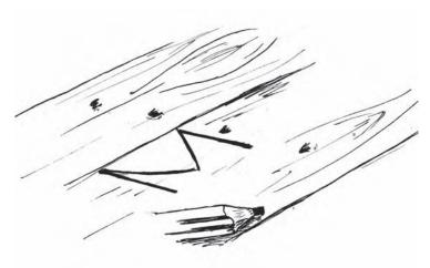
Figure  ${\bf 6.3}\,$  Pencil markings on the floor to indicate the position of the bottom of a timber framed wall
