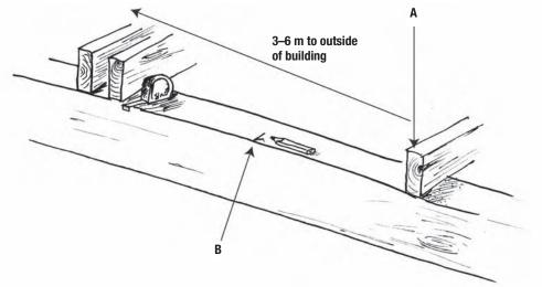
Figure 3.8 Mark the bearer for floor joist positions
