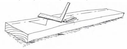
Figure 17.5 Marking the stringer with the tread positions
