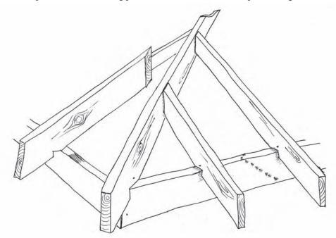
Figure 8.31 45-degree angle cut at the top of the creepers to enable fixing them to the face of the hip beam
