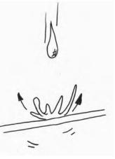
**Figure 9.2** The energy of rain striking a flat roof is transferred to the roofing material, thereby resulting in increased noise
