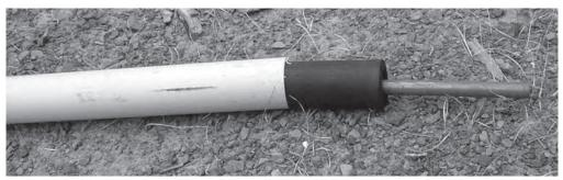
Figure 13.2 Copper pipe covered with black foam in a PVC pipe
