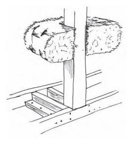
Figure 5.16 Securing of a load bearing post to the floor via bottom boxing
