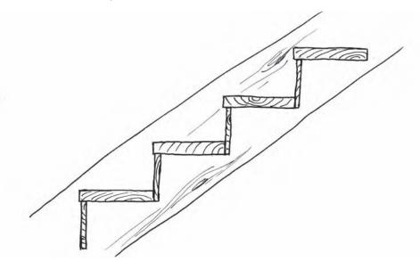
Figure 17.2 Sectional view of a staircase with the tread overhanging the riser by 10 mm
