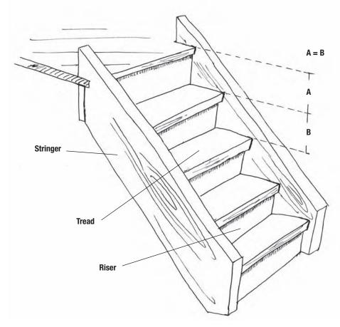
Figure 17.6 All risers of a staircase are to be equal
