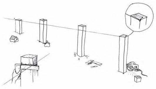
Figure 3.4 String line to ascertain the cut off point of timber stumps
