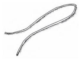
Figure 4.8 Wire pins are used to secure the compression strapping to the straw bales
