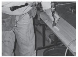
Figure 14.6 Chisel held vertically to cut the clean edge of the hinge checkout
