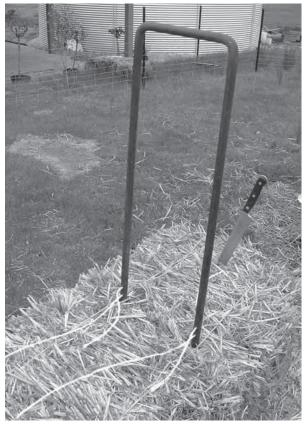
Figure 4.14 Twine is fed through the eyes of the needle for later tying of the new length bales
