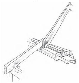
Figure 8.14 Installation of rafters for the main roof and the verandah, coupling them together at the top boxing
