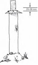
Figure 3.5 The application of skew nailing
