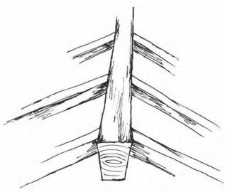
Figure 8.24 Pairs of rafters are to be fitted directly opposite one another at the ridge
