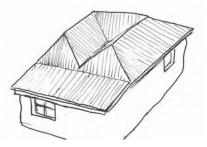
$\pmb{8.7}$  'U' shaped roof with a box gutter and a leant to extension
