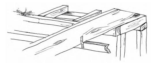
Figure 7.6 Installation of a hanger with an angle cut supported on a jack joist
