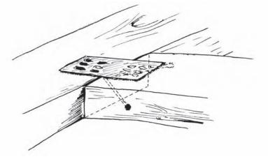
Figure 6.17 Joining of wall junctions at the top wall plate using a nail plate and two skew nails
