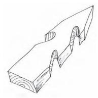
Figure 4.21 Barbed timber peg to be hammered into the straw bale wall
