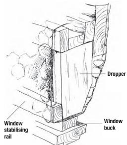
Figure 5.10 Dropped rolled head for infill construction
