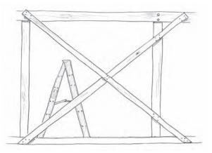
Figure 4.20 Temporary braces are used to stabilise the frame until after the straw bales are installed and connected to the frame
