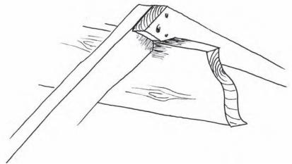
Figure 8.15 Installation of a pair of rafters onto a load bearing ridge
