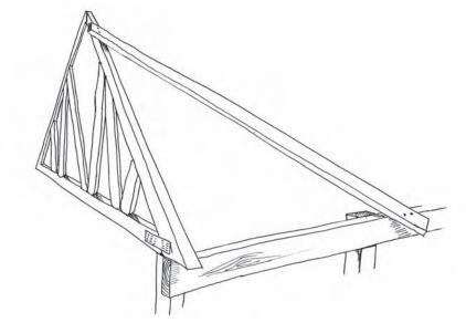
Figure 8.34 Initial securing of the first truss installed, using a temporary angle brace
