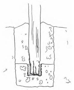
Figure 3.2 Timber stumps encased in concrete can lead to the degradation of the stump
