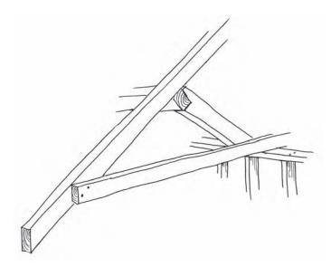
Figure 8.17 Installation of underpurlin and struts to provide mid-span support of rafters
