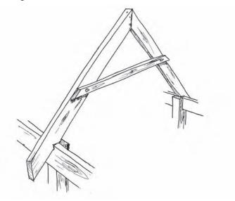
Figure 7.7 Collar tie bolted to the rafters to create a barn shaped ceiling
