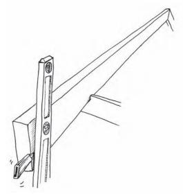
**Figure 9.3** Marking the tail of a rafter to be cut in preparation for the installation of the fascia
