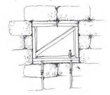
Figure 5.8 Small window buck with an internally fitted diagonal brace, installed into a straw bale wall
