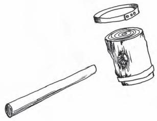
**Figure 4.7** Bales protruding beyond the desired line of the wall are re-positioned using a bale hammer
