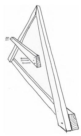
Figure 8.33 Installation of a collar tie to the sides of a pair of rafters in a coupled roof
