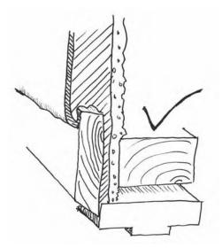
**Figure 10.7** Render that finishes on the vertical face of the window head architrave will discharge water cleanly from the render
