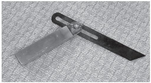
Figure 8.28 Adjustable bevel
