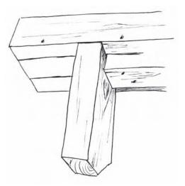
Figure 5.9 Droppers and nogging for dropped rolled head secured to the underside of top boxing
