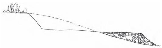
Figure 2.3 Cut and fill site preparation
