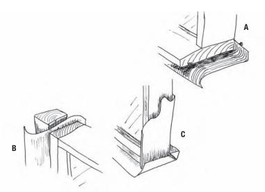
Figure 10.3 A side flashing for a timber window. Note that the sill flashing is to envelope the side flashing at their junction
