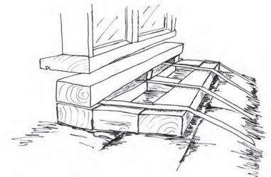
Figure 5.11 Compression timber beneath a non-centrally located window
