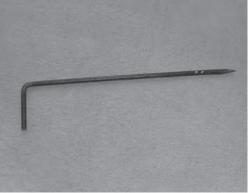
Figure 4.11 Double bale needle used for cutting special length bales
