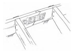
Figure 8.26 Joining of a ridge beam with 45-degree angle cuts and nail plates
