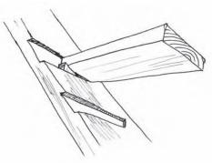
Figure 17.3 Installation of a tread into the checkout in the stringer with the use of a wedge
