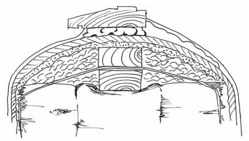
Figure 10.8 Expanding foam sealant in the installation of a window at its sill
