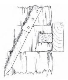
Figure 5.3  $190 \times 45$  door buck with  $70 \times 45$  stiffening and bale stabilising rib
