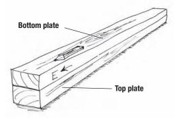
Figure 6.8 Marking the sides of the bottom wall plates to assist in the relocation of the wall onto the floor for assembly
