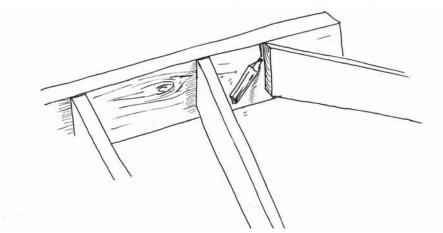
Figure 8.27 Marking the cut off position of the ridge for the installation of the last jack rafter
