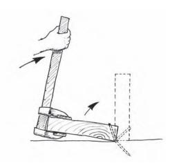
Figure 7.3 Angle nailing of the hanger to the ceiling joists
