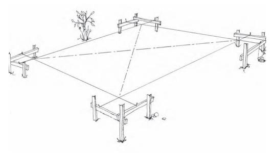
Figure 2.7 Check the diagonals of the setout to ensure the building is square
