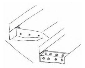
Figure 17.4 Metal and timber mounting blocks fixed to the stringer to support the treads
