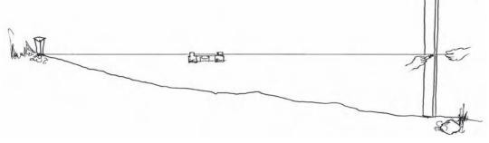
Figure 2.1 String line level to establish the basic fall in the building site
