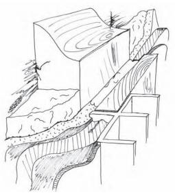
Figure 10.9 Installation of an aluminium window using expandable foam sealant
