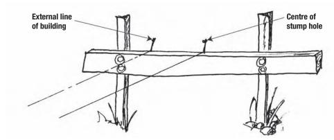
Figure 2.5 Profile hurdle for the location of the stump holes and the outside line of the building
