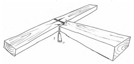
Figure 6.4 Marking the junction of three timber-framed walls
