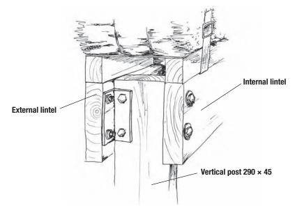
Figure 5.17 Double lintel fixed to  $290 \times 45$  post to support straw bales over a wide opening
