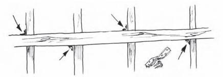
Figure 7.2 Plan view of joist straps at the junction of the hanger and ceiling joists
