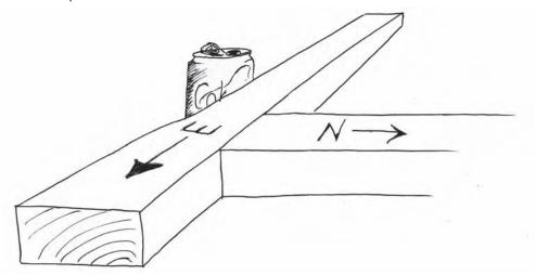
Figure 6.5 Markings to indicate the direction of timber framed walls
