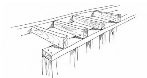
Figure 7.1 Installation of jack joists from the ceiling joist to the top of a parallel wall
