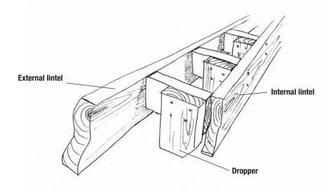
Figure 5.18 Noggings and droppers fixed to double lintels
