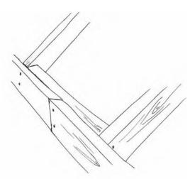
Figure 9.4 Joining fascia over a nogging between two rafters
