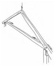
**Figure 8.10** Rafters supported by a load bearing central ridge beam held up by posts, and by pitching beams on posts at the outside walls
