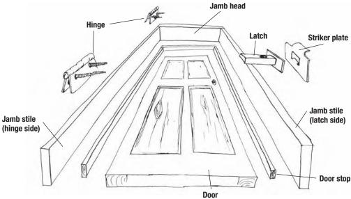
Figure 14.1 The components of a door jamb
