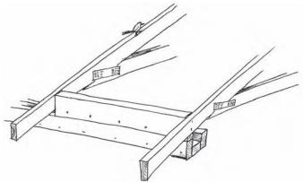
Figure 4.19 Securing the timber infill frame to the straw bale walls using  $190\times45$  rafter blocks
