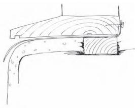
Figure 10.4 Sill flashing fixed to facilitate water discharge onto the external face of the rendered wall below the window
