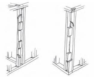
Figure 6.19 Fixing of wall junctions up the length of the stud
