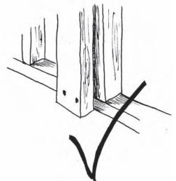
**Figure 6.7** Installation of a door stud 45 mm longer than a standard stud to negate the need for a short section of bottom wall plate beneath the stud
