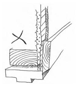
Figure 10.6 Render that finishes on the horizontal surface of a window head architrave is likely to result in deterioration of the render at that junction
