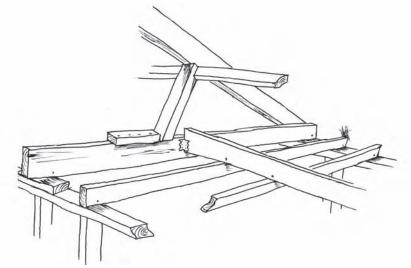
8.22 Strutting beam onto the top of two walls to support a hanging beam and strut to the underpurlin
