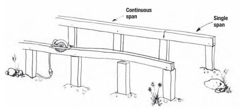
Figure 3.6 Crippling the bearer reduces it to a single span and reduces its span capacity
