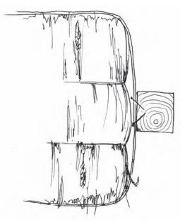
Figure 5.2 Wire netting fixed to the back of the door buck and over the straw bales
