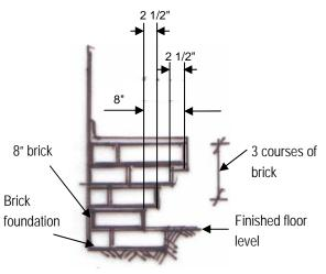
Fig 5 - Section at corbel seat
