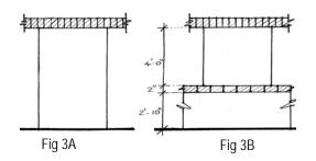
It is important to ensure that the row of bricks serving as a base for lintels placed at the top of door and window openings should extend not less than 6" inches beyond the sides of the opening as shown in **fig** 3A and 3B.
