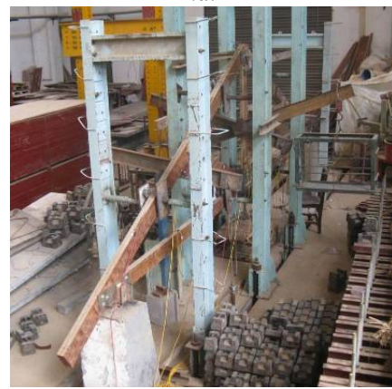
Figure 13: Glulam truss test: (a) loading condition; (b) test setup
