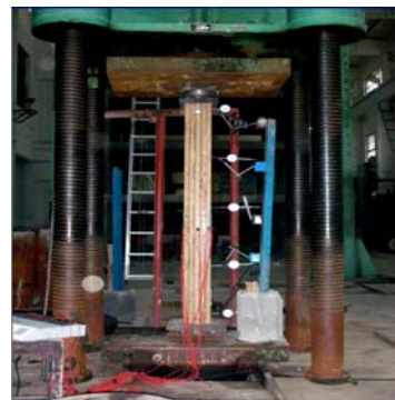
Figure 11: Test setup for glulam columns
