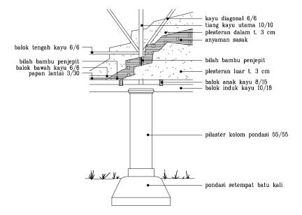
They used wooden skeleton and bamboo woven mat in the outer skin before plastered. The wooden frame could be seen from the interior, but the exterior had an image of brick wall construction.
