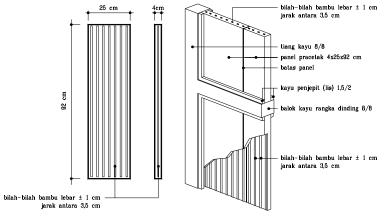
The detail of bamboo splits reinforcement in precast panels (left).
