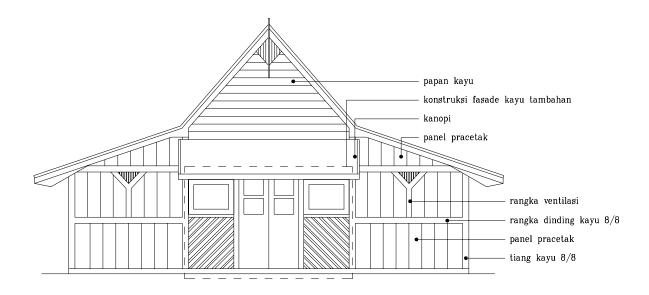
Front elevation of Gempol House. Precast concrete with bamboo reinforcement dominated the façade. Built in 1923, these 101 houses used to accommodate local colonial government employee in
