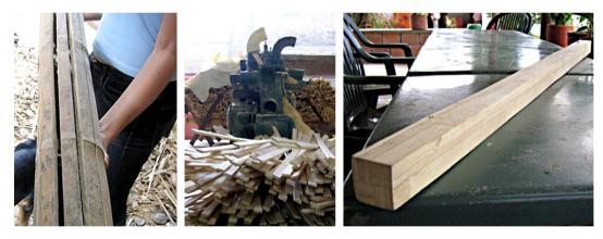
Fig. 1. From round bamboo to bamboo strips ('latas') to laminated bamboo beam/column. Source: Juan Ayala.
