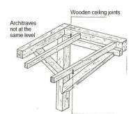
Figure 4d. Top view of correct positioning for architraves.
