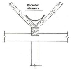
Figure 3a. Wrong way to build a trough gutter.
