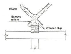
Figure 3b. Correct way in which to build a trough gutter using bamboo rafters.
