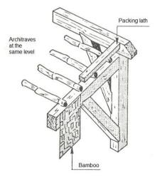
Figure 4c. Top view of correct positioning for architraves.
