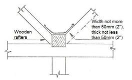
Figure 3c. Correct construction of trough gutters using wooden rafters.
