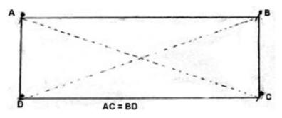
Figure 3: Initial foundation layout
