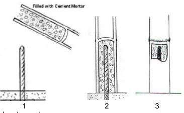
Figure 6: Fixing bamboo column
