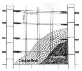
Figure 8: Wall structure
