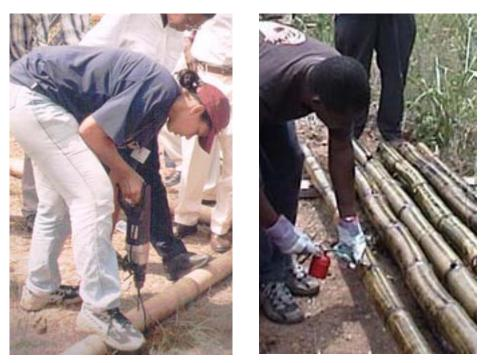
Pictures 1-2: Drilling and Injecting Creosote Oil
