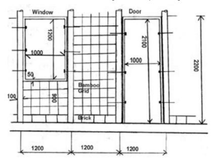
Note: Door or window frames must be hanged before plastering the walls.
