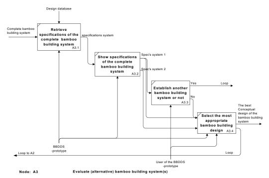
Figure B.12: Evaluate (alternative) bamboo building system(s)
