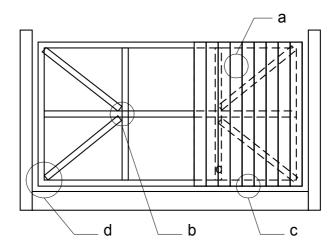
Figure 5.9: Types of connections on the wall
