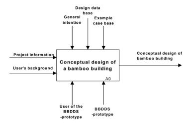
Figure 4.2: Main activity of the conceptual design of a bamboo building
