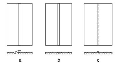
Figure 5.10: Connection between wall-fillers
