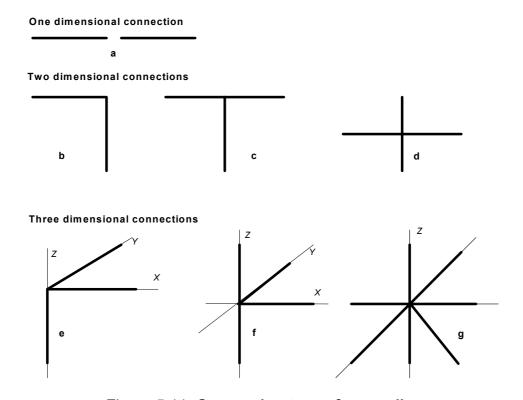
Figure 5.11: Connection types for a wall
