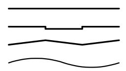
Figure 5.8: Typical forms of a bamboo wall
