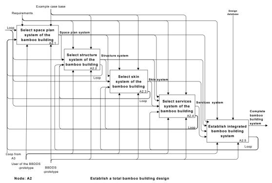
Figure B.6: Establish a total bamboo building design
