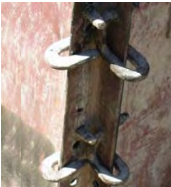
Four clamps mounted in edge-position using an angle bar
