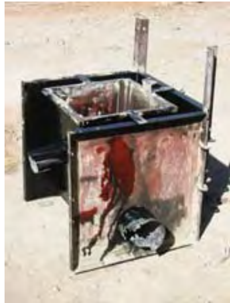
The mould viewed from the side of the catch drain (front panel removed)
