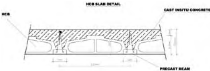
Fig-4s section of slab at final condition
