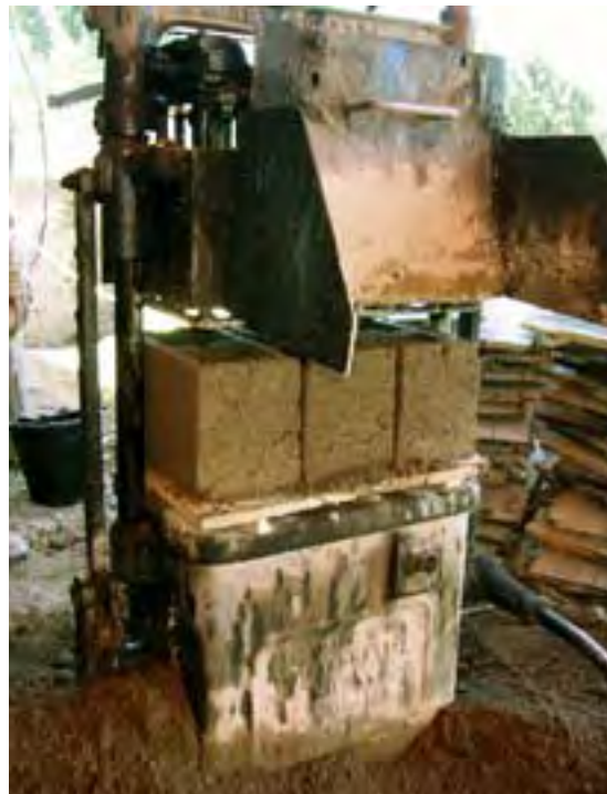
Removing the mould upwards
