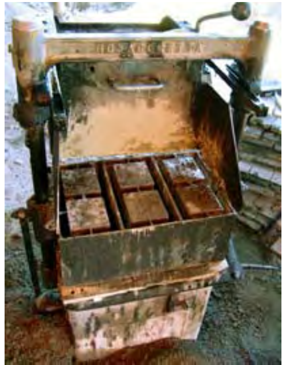
The machine used for the production of HCBs
