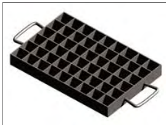
The mould for the concrete spacers
