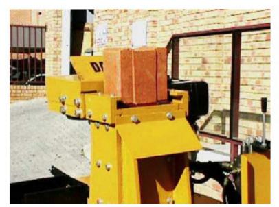
After compaction of the Low Cost Housing brick a second lever is pressed to press the brick from the machine giving a durable, waterproof brick for building.
