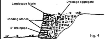
stone walls 2-1/2 Feet and under, elaborate drain systems are not necessary, although landscape fabric is still necessary to stop soil on the slope from washing through the wall creating erosion above and behind
