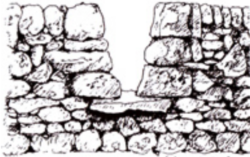
One type of squeeze style. (Image: Dry Stone Walling, Techniques and Traditions, 2004)
