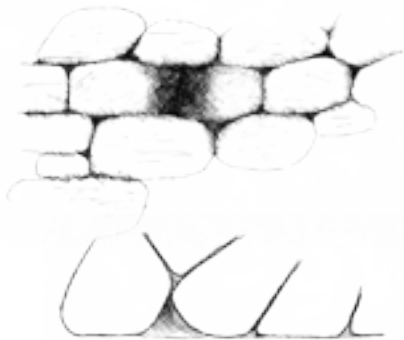
Elevation and plan of a stone with a curved face that is not aligned well.
