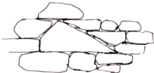
This is correct, with stones set so that the bottoms are level.
