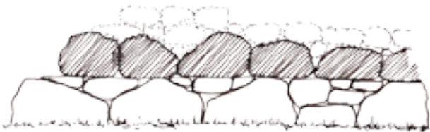
After placing the footings, the wall is built to a level plain. Then the large stones (hatched) are put on, then the wall is built normally on top (dashed).
