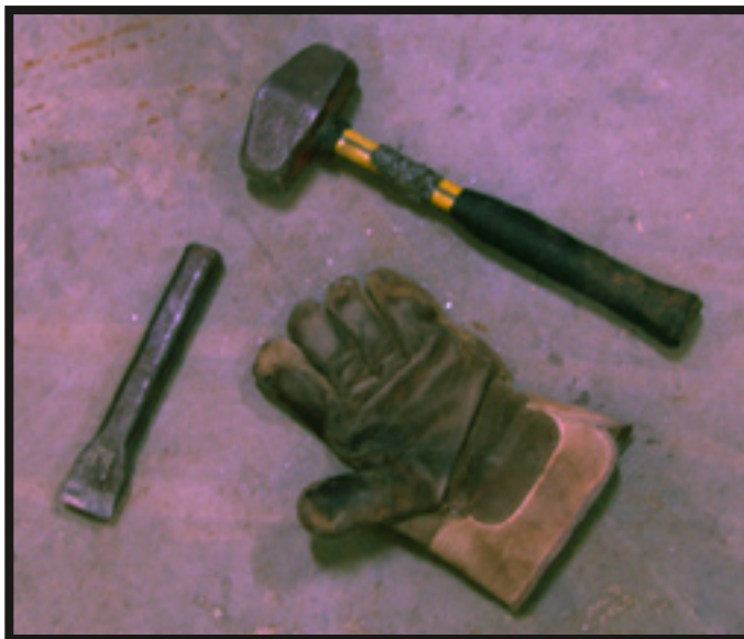
A three pound lump hammer with a tracing chisle and glove for scale.
