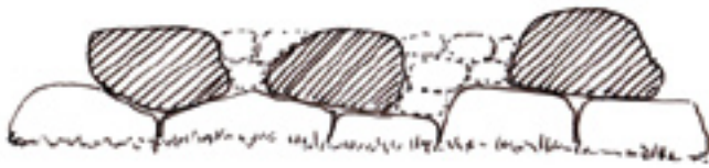
After placing the footings, the largest stones left (hatched) are placed and then the wall is built up in between (dashed).
