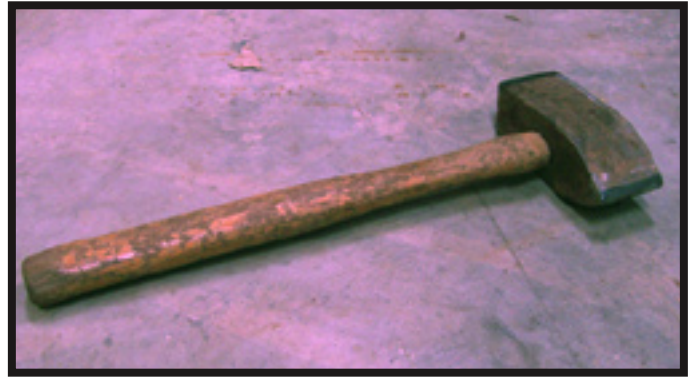
A walling hammer with a carbide-tipped head.
