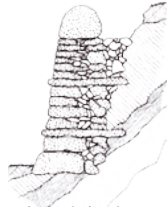
Section of a single faced retaining wall. (Image: Dry Stone Walling, Techniques and Traditions, 2004)
