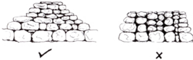
A well built wall with all joints crossed on the left. An extreme case of running joints on the right. (Image: Dry Stone Walling Techniques and Traditions, 2004)
