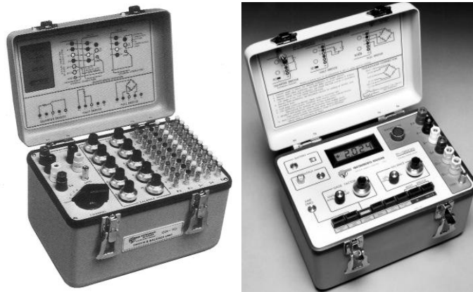
Figure 63: SB-10 Switch & Balance Unit and P-3500 Digital Strain Indicator
