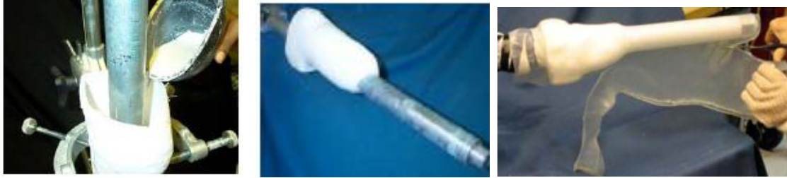
Figure 5: Pouring Plaster into Limb Casting, Mandrel with Positive Mold, and Cutting the Plastic (CIR 2006)
