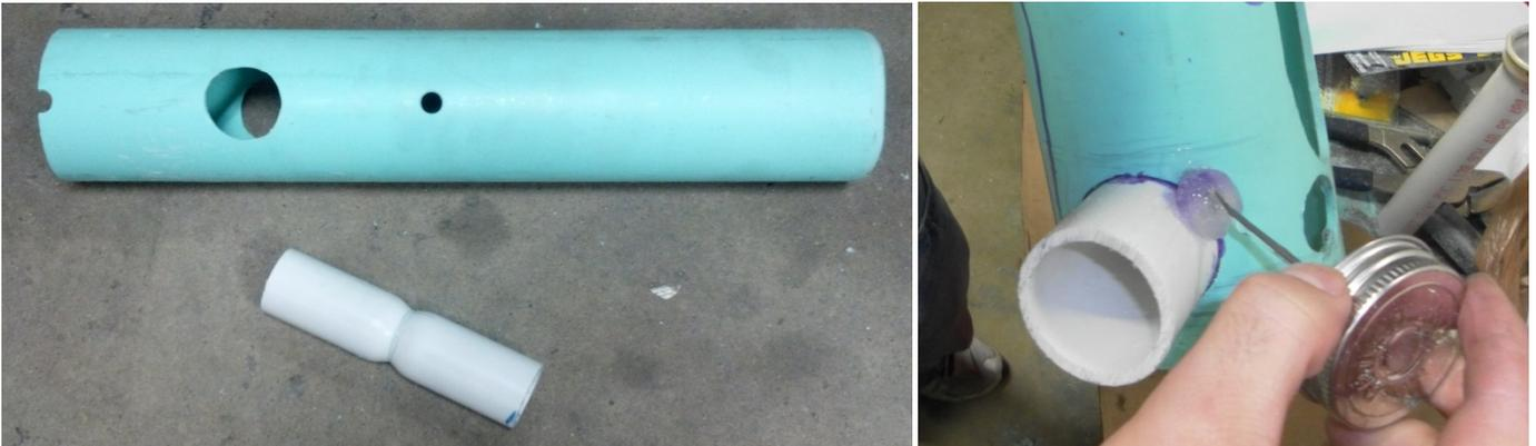
3) Locate 10" length of PVC pipe with same diameter as rising pipe. Using PVC primer and cement, secure the coupler (#6 in picture) to one end of the rising pipe (#7 in picture). Allow to dry completely.
