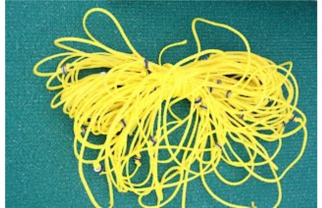
Strength is not an issue because it is extremely rare for a pump rope to handle more than 10 pounds.
