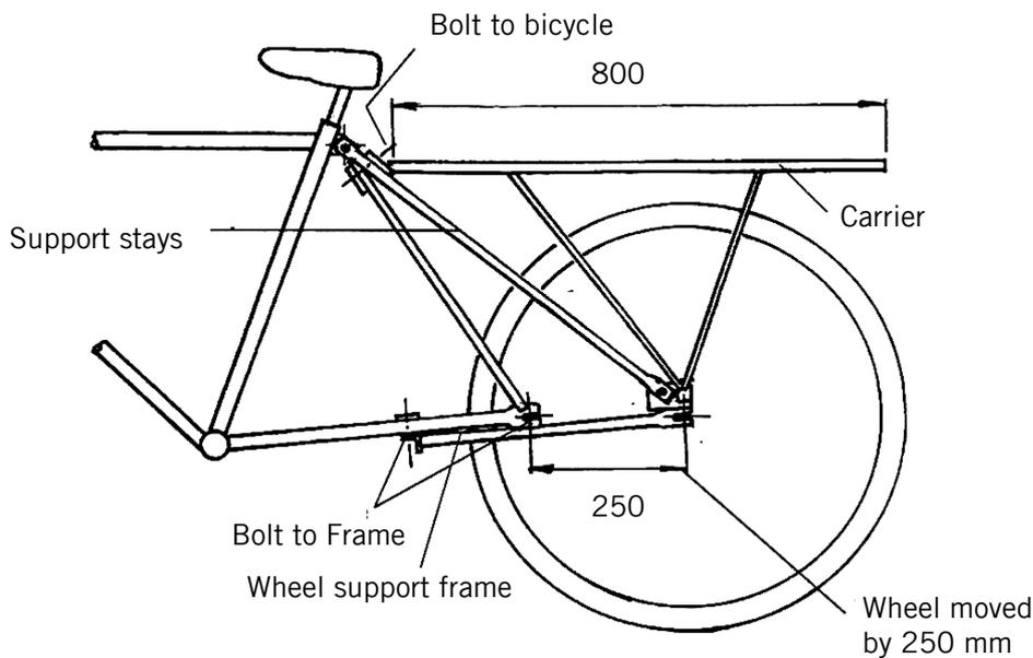
Figure 4: Construction of extension for a standard bicycle
