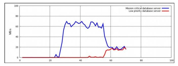
Figure 4.1. I/O throughput without resource allocation
