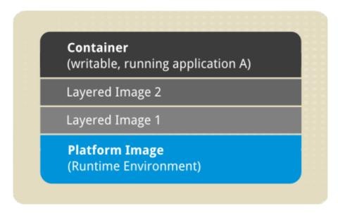
Figure 5.4. Image Layering Using Docker Format
