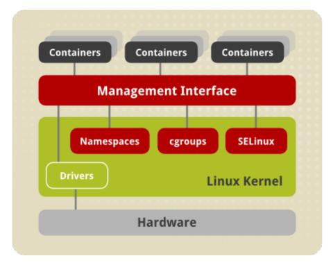
Figure 5.1. Linux Containers Architecture
