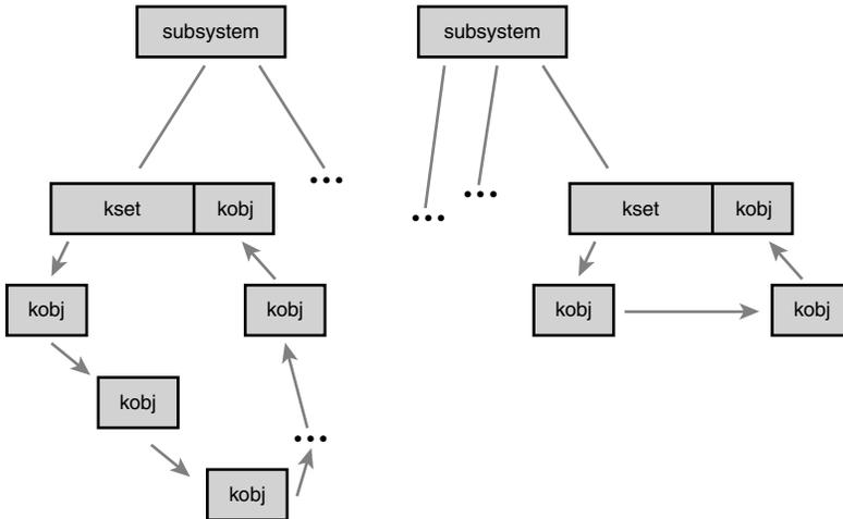
Figure 17.1 Relationship between kobjects, ksets, and subsystems.
