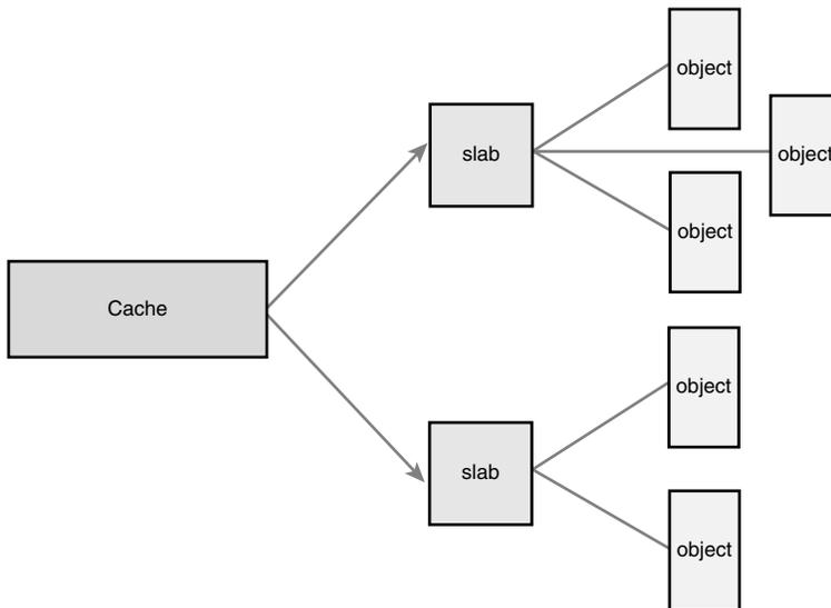
Figure 12.1 The relationship between caches, slabs, and objects.
