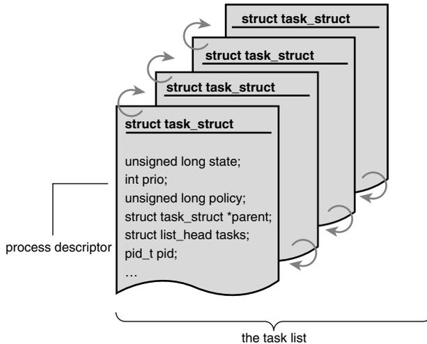
Figure 3.1 The process descriptor and task list.
