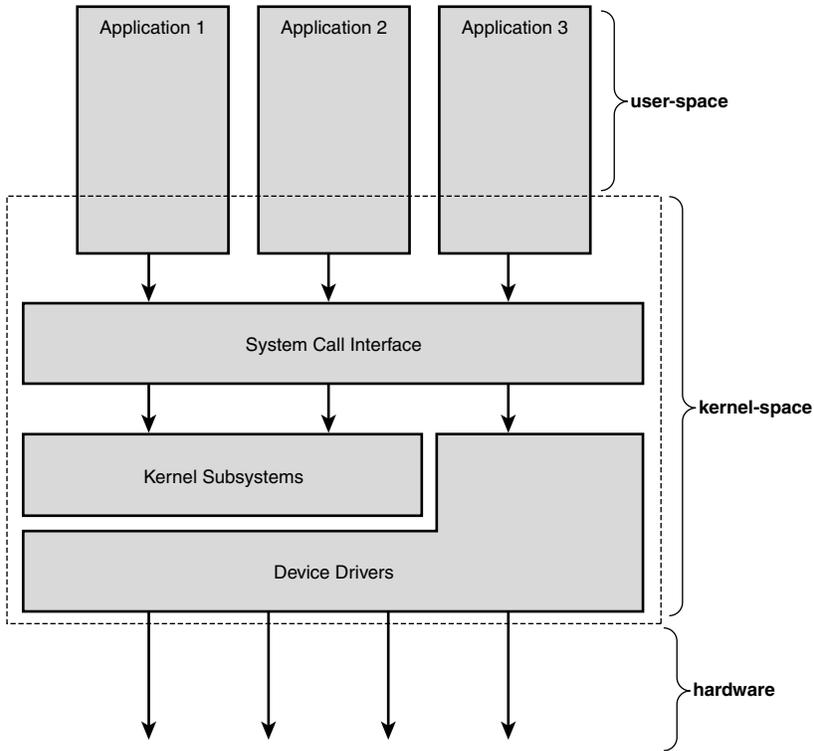
Figure 1.1 Relationship between applications, the kernel, and hardware.
