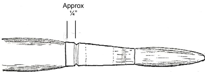
Figure A6: Fitting handle to ferrule
