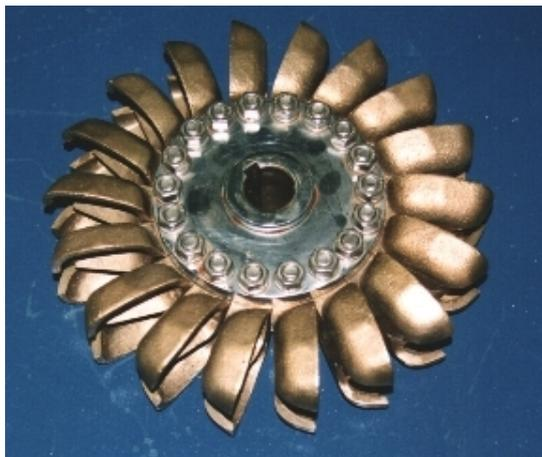
Figure 8-5 Locally Manufactured Pelton p.c.d.180 mm (Sri Lanka)
