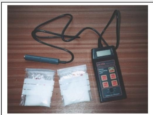
Figure 7-7 Portable conductivity meter and carefully weighed bags of salt
