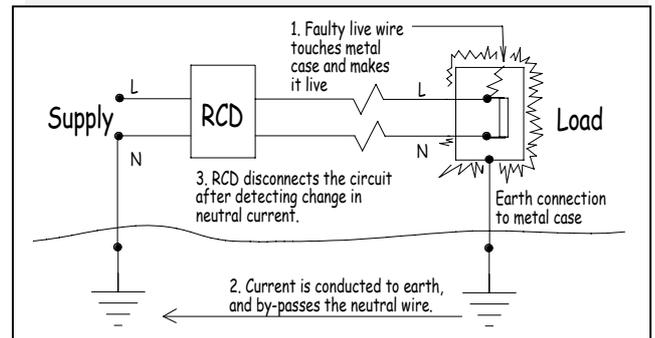
Figure 15-4 Protecting consumer loads using an RCD
