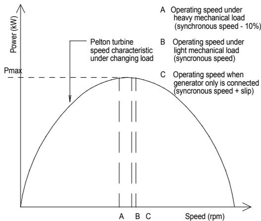
Figure 19-7 Ideal operating speeds of Pelton turbine under different load conditions
