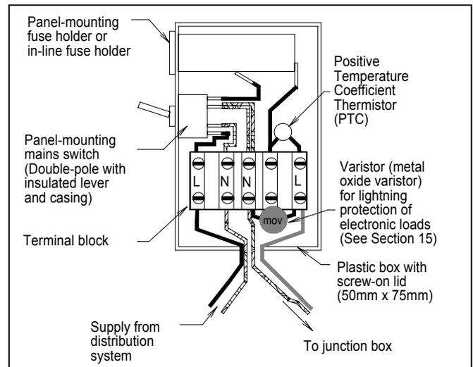
Figure 15-7 A load limiter should connect the service wire from the distribution system to the domestic wiring in the house. A PTC is used as a load limiter if less than 0.5 Amps is drawn.
