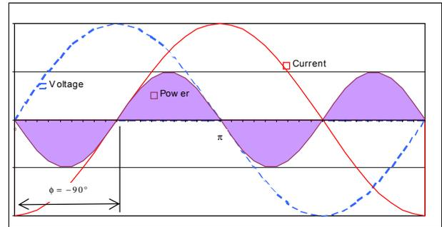
Figure 19-4 If the load is a pure inductor, then the current lags the voltage by 90°. The average power consumed is still = 0 Watts
