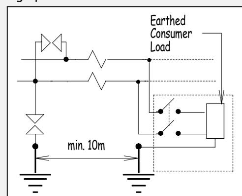
Figure 16-3 Ensure that the consumer earth electrode (if used) is at least ten metres from the neutral-earth arrestor electrode.
