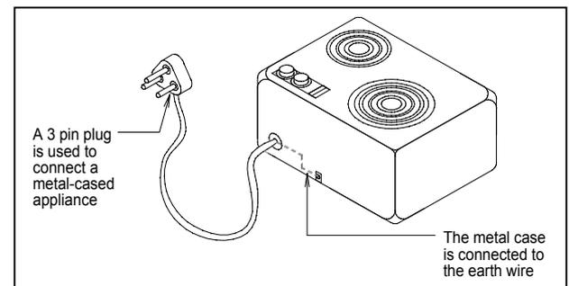
Figure 15-5 Metal-cased devices should be earthed
