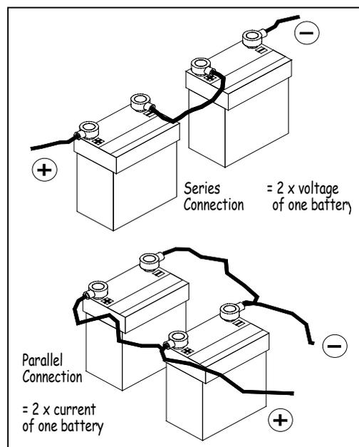
Figure 19-1 Series and parallel connection of batteries
