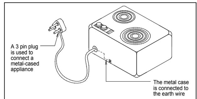
Figure 15-5 Metal-cased devices should be earthed
