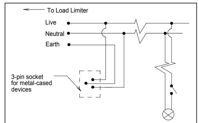
Figure 15-6 An earth connection must be provided if metal cased loads are likely to be connected.
