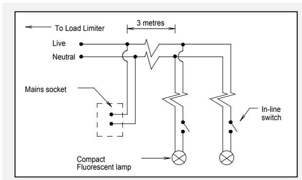
Figure 15-3 Circuit diagram of a typical wiring harness
